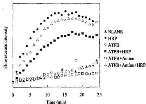
Fig. 4 Time course of the fluorescence intensity of Resorufin by the HRP-catalyzed oxygenation of Amplex Red.
