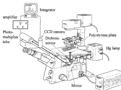
**Fig. 2** Schematic diagram of microscopic fluorescence imaging system used for confirmation of immobilization of Avidin488.
