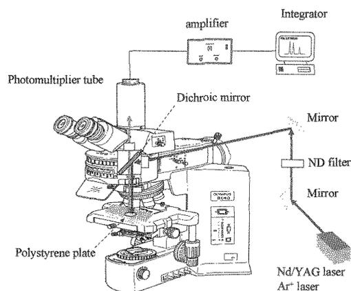
**Fig. 1** Schematic diagram of microscopic fluorescence analysis system used for confirmation of immobilization of HRP and ALP.
