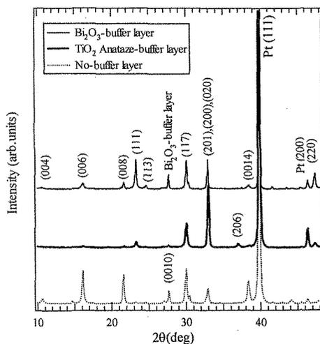
Fig.4 XRD patterns of as-deposited BIT thin films with no-buffer layer, TiO<sub>2</sub> Anataze-buffer layer, and Bi<sub>2</sub>O<sub>3</sub> buffer layer.
