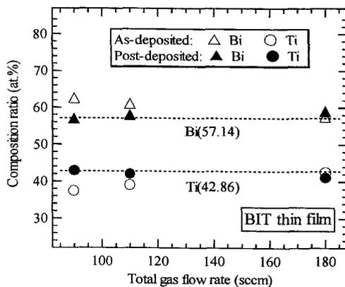
Fig. 1 Comparison ratio of composition ratio between as-deposited and post-annealed BIT thin films deposited at total gas flow rates of 90, 110, and 180 sccm.
