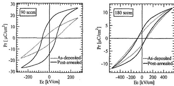
Fig. 3 Comparison of *P-E* hysteresis loops between the as-deposited and post-annealed BIT thin films deposited at 90 and 180 sccm.
