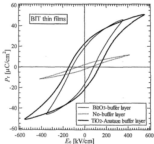
Fig. 5  $P$ - $E$  hysteresis loops of as-deposited BIT thin films with no buffer layer,  $\text{TiO}_2$  Anatase buffer layer and  $\text{Bi}_2\text{O}_3$  buffer layer.
