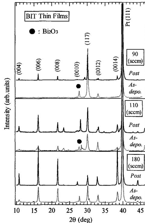
Fig. 2 Comparison ratio of the XRD patterns between as-deposited and post-annealed BIT thin films deposited at total gas flow rates of 90, 110, and 180 sccm.
