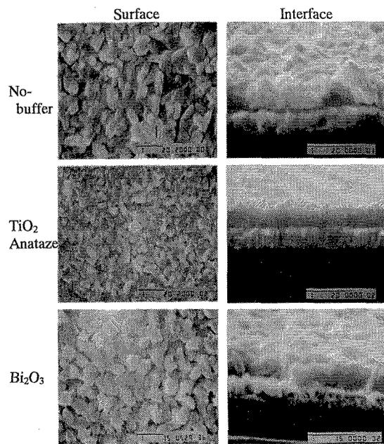
Fig. 5 Surface morphologies and SEM cross-sectional micrographs of as-deposited BIT thin films with no buffer layer, TiO<sub>2</sub> Anataze-buffer layer and Bi<sub>2</sub>O<sub>3</sub> buffer layer.
