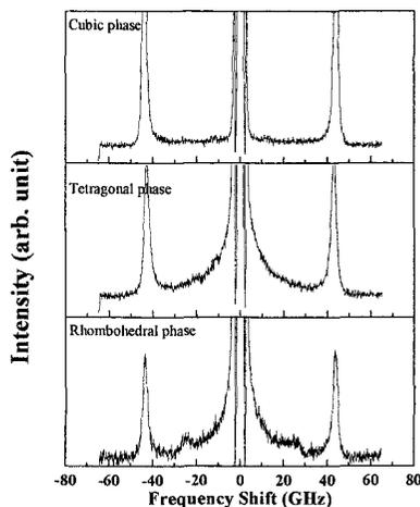
Fig. 2 Brillouin spectra obtained at the backward scattering geometry
