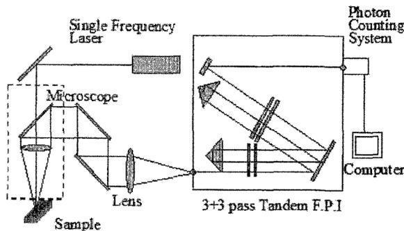
Fig. 1 The Brillouin scattering system with a tandem Fabry-Perot interferometer
