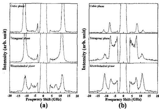
Fig 3. The Brillouin spectra at the right angle scattering geometry. (a) VV and (b) VH spectra
