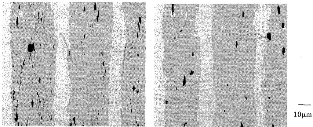
Figure 2. SEM image of (a) 0.1 MPa sintered sample and (b) pressure sintered sample. The gray regions, black regions, white regions and tiny irregular black regions are Bi2223, alkaline earth cuprates (AEC), Ca-Pb-O and pores, respectively.
