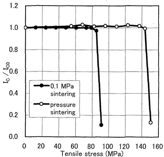
Figure 6. Tensile stress tolerance of 0.1 MPa sintered sample and pressure sintered sample.  $I_c$  and  $I_{c0}$  mean critical current after tensile stress and without tensile stress, respectively.
