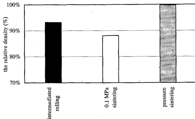
Fig.1. The relative density of Bi2223 wires with intermediated rolling process, 0.1 MPa sintering process and pressure sintering process.
