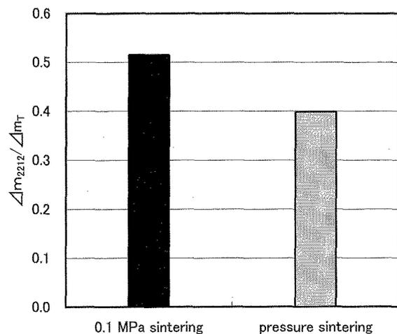
Figure 4. Bi2212 content in filaments from DC magnetization curves in fig. 3.
