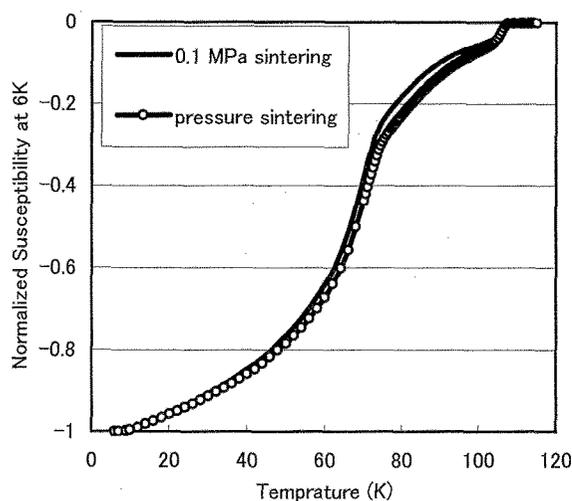
Figure 3. DC magnetization curves of 0.1 MPa sintered sample and pressure sintered sample using SQUID. Magnetic field of 10G applied parallel to the wire surface.
