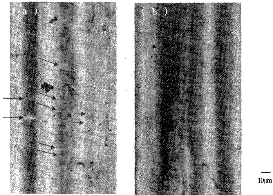
Figure 5. Magnet-Optical image of (a) 0.1 MPa sintered sample and (b) pressure sintered sample at  $T=10$  K and  $H=800$  G. The parts indicated by arrows are defects.
