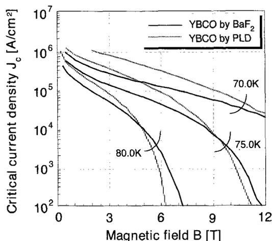
Fig. 1 Critical current densities vs magnetic fields for the YBCO film prepared by no-additional-water annealing of precursor film and the PLD-YBCO films.
