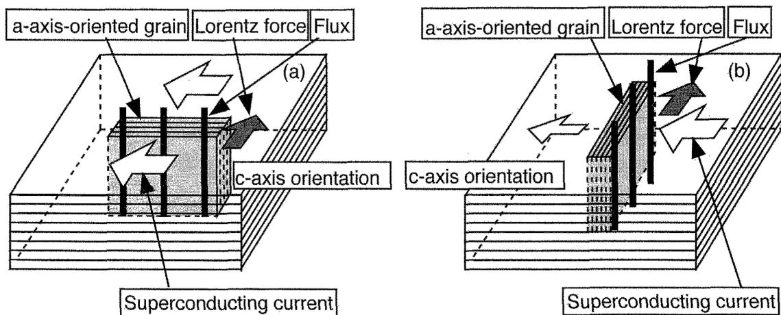
Fig. 4 Conceptual models of the pinning centers along to the c-axis direction (a) and the interrupt of superconducting current flow (b).
