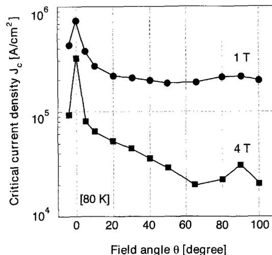
Fig.2 Field angle dependences of the critical current density at 80 K in 1 T and 4 T.
