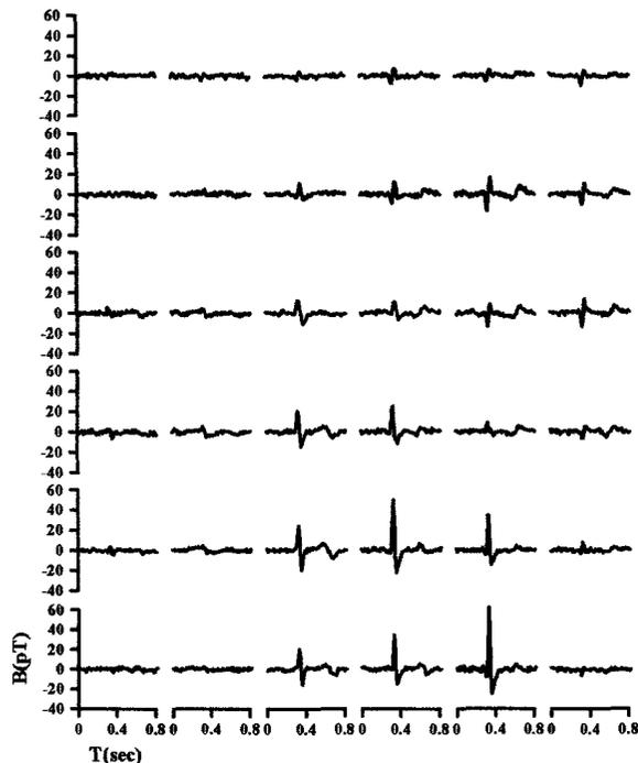
Figure 5 Averaged MCG signals measured at 36-points on the sensing plane above the thorax of the subject.
