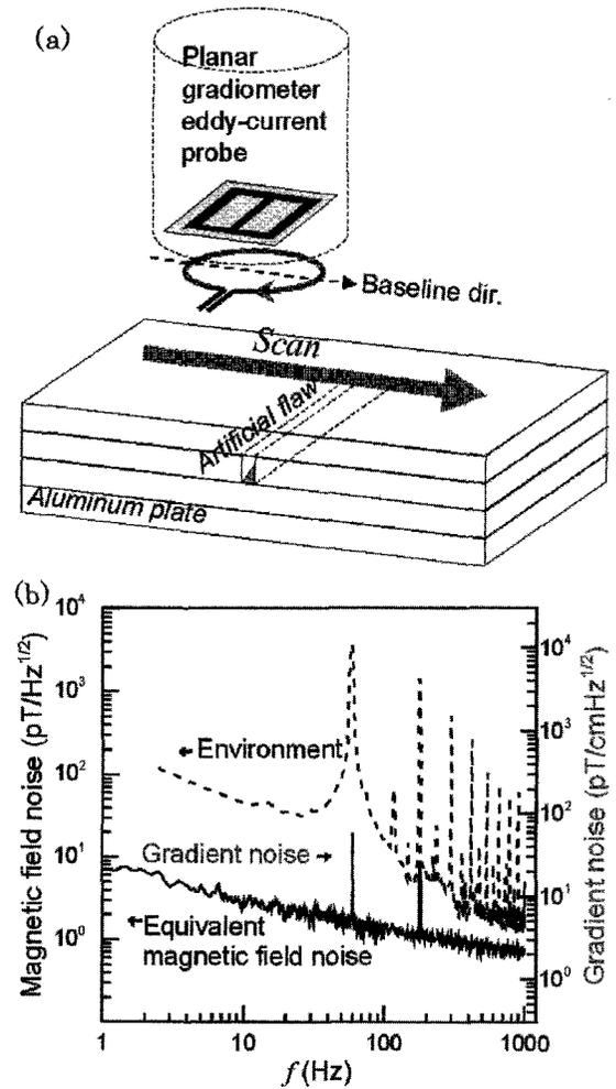
Figure 2 (a) Planar SQUID gradiometer eddy-current probe with a circular excitation coil. (b) The gradient noise and the equivalent magnetic noise of the gradiometer.
