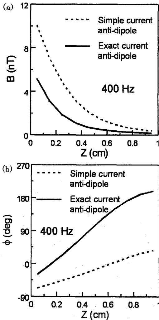
Figure 3 (a) The magnitude, and (b) the phase, of the defect signal of the simple current anti-dipole and the exact current anti-dipole.  $Z$  is the depth of the current anti-dipole.
