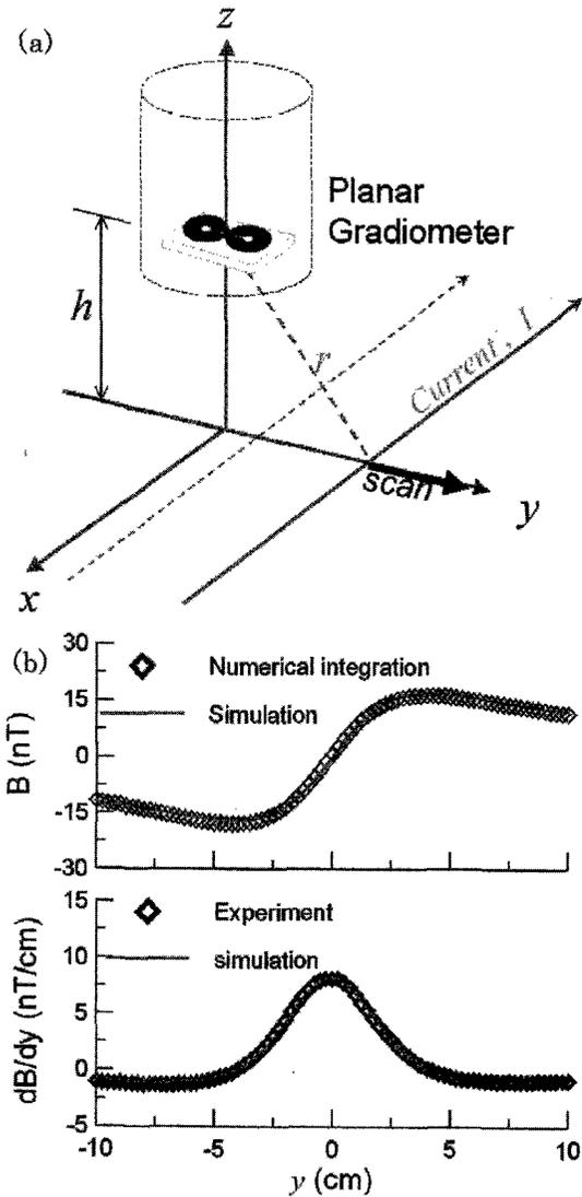
Figure 1 (a) Calibration of the gradient-to-voltage transfer function of the planar gradiometer by measuring the magnetic field gradient map of a long-straight current carrying wire. (b) The magnetic field gradient map measured with the planar gradiometer is transferred into the magnetic field map by means of a numerical integration technique.
