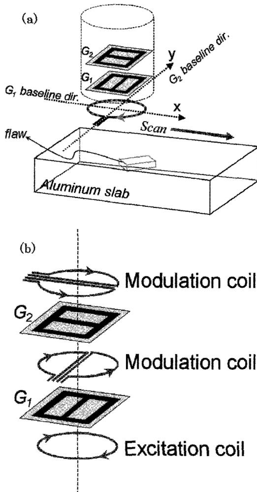
Figure 5 (a) Orthogonal planar SQUID gradiometers eddy-current probe with a circular excitation coil, the probe is sensitive to in-plane oriented flaws. (b) Modulation schemes for the orthogonal planar gradiometer eddy-current probe.
