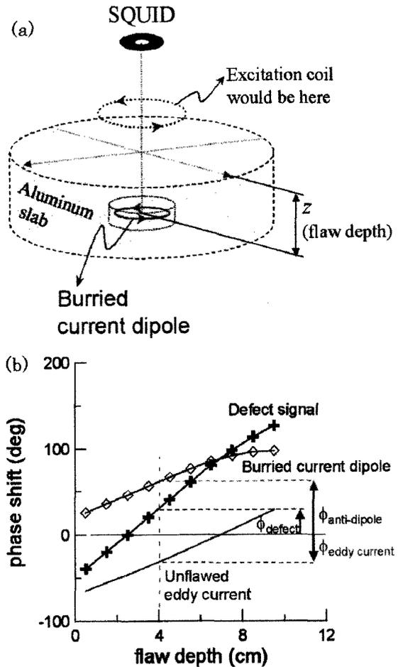
Figure 4 (a) Experimental set-up for measuring the phase shift of the magnetic field for a buried dipole, (b) phase shift of the magnetic field with respect to the buried current dipole (+), phase shift of the unflawed eddy current (solid line), and the phase shift of the defect signal (diamond). The frequency is 400 Hz.
