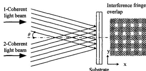
Fig.3 The interference fringe and their overlay of coherent light in interference field of substrate
