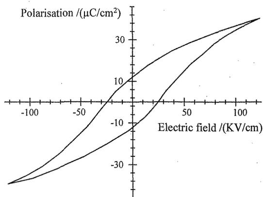
Fig.9 The curve of hysteresis loop of PZT film
