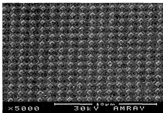
Fig.6 SEM photo the combinative structure pattern with dot array and lattice of PZT film
