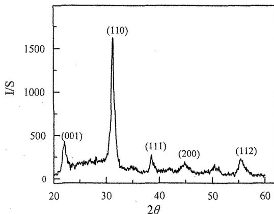
Fig.8 XRD diffraction patterns of the PZT films
