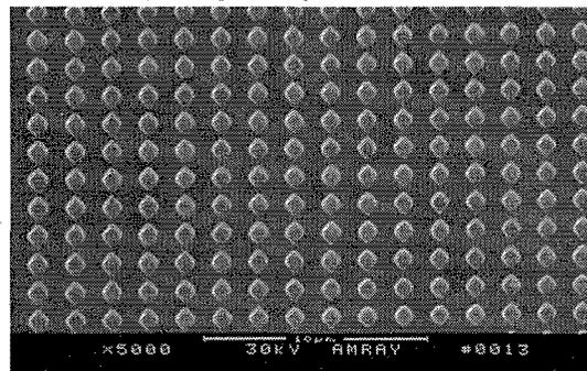
Fig.5 SEM photo of the dot array structure pattern of PZT film
