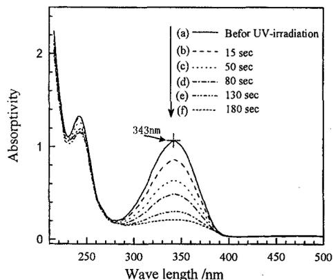
Fig.1 The ultraviolet spectrum absorption peak of PZT gel film and its intensity variation under the ultraviolet light irradiation
