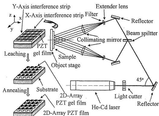
Fig.4 The schematic diagram of PZT film fine patterning by double interference exposure with two beam ultraviolet laser
