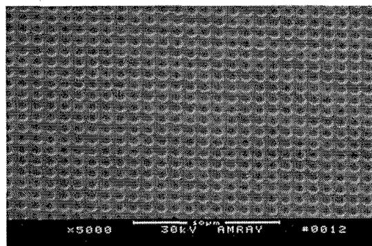
Fig.7 SEM photo of the lattice structure pattern of PZT film
