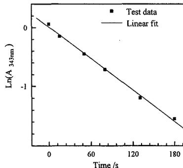
Fig.2 The relationship between intensity of absorption peak at 343nm of PZT gel film and the time of ultraviolet light irradiation
