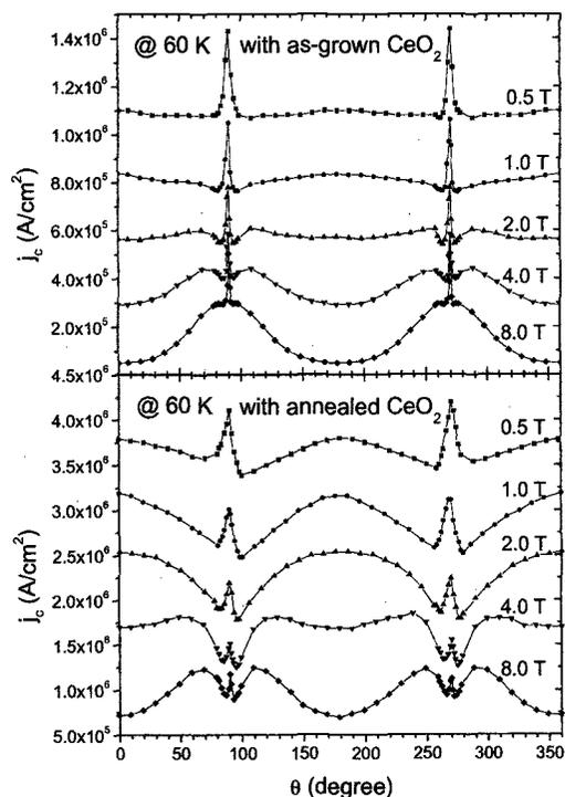
Figure 3. Critical current density  $j_c$  at 60 K as a function of angle  $\theta$  between the applied magnetic field (H) and the film normal. Two typical films deposited on R-cut sapphires with the as-grown and the annealed CeO<sub>2</sub> buffer layers were measured and compared.
