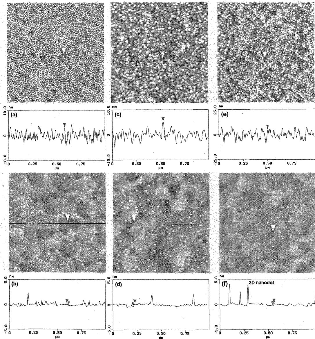
Figure 1. AFM images of three  $\text{CeO}_2$  films with thicknesses of (a) (b) 10.0 nm, (c) (d) 23.6 nm and (e) (f) 36.6 nm, respectively, on R-cut sapphire substrates before and after the high temperature  $\text{O}_2$  annealing.
