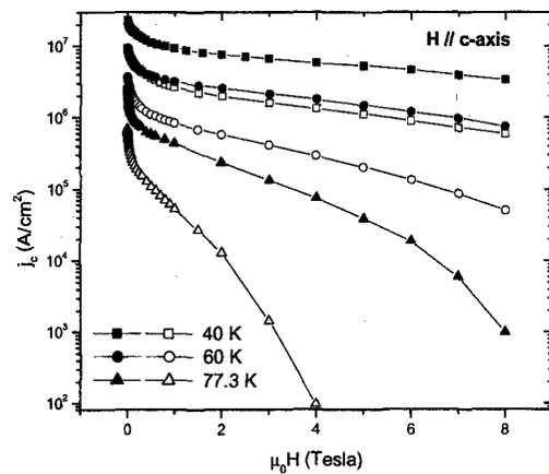
Figure 2. Critical current density  $j_c$  as a function of applied magnetic field (H) at various temperatures for two typical 200-nm-thick YBCO films on R-cut sapphire with a 36-nm-thick annealed (solid) and as-grown (open) CeO<sub>2</sub> buffer layer, respectively.
