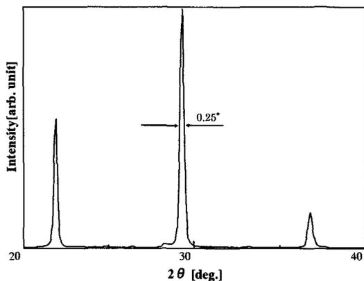
**Fig. 2** XRD pattern of the film prepared at 830°C using the target of Bi:Sr:Cu = 6.0:1.8:0.6
