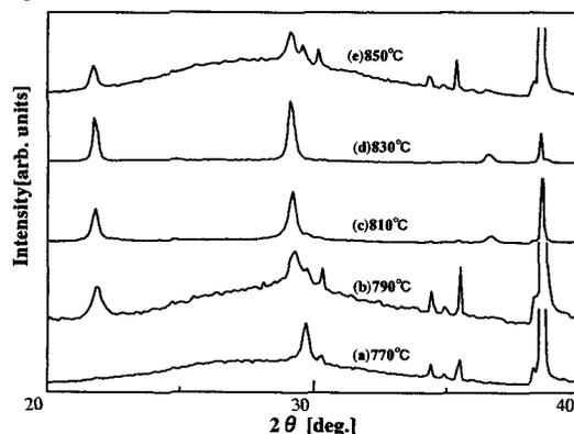
**Fig.1 XRD patterns of the films prepared at various substrate temperatures (*T<sub>sub</sub>*) using the target of Bi:Sr:Cu = 4.8:2.1:0.6**
