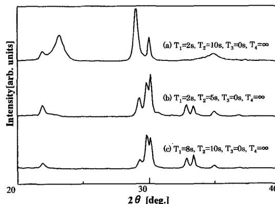
**Fig. 5** XRD patterns of the films prepared at 830°C using two targets of Bi-Sr-Cu-O and Ca-Cu-O with various the shuttering conditions of (a), (b) and (c)
