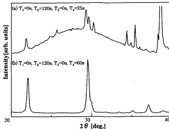
**Fig. 4** XRD patterns of the films prepared at 830°C using two targets of Bi-Sr-Cu-O and Ca-Cu-O with different shuttering conditions of (a) and (b)
