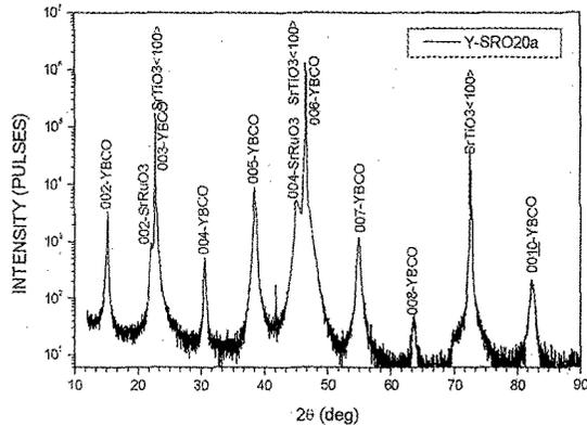
Fig.1. X-ray diffraction pattern of a (80nm/20nm)<sub>5</sub> YBCO/SRO superlattice.
