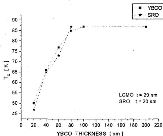
Fig.4 Evolution of  $T_C$  as a function of the YBCO thickness in YBCO/LCMO and YBCO/SRO superlattices with  $t_{\text{LCMO/SRO}} = 20\text{ nm}$ .
