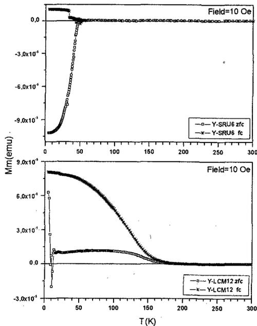
Fig.7 Zero field cooled ( $\square$ ) and field cooled ( $\xi$ ) magnetization vs. temperature plots for an YBCO/SRO (20nm/20nm)<sub>10</sub> (top) and an YBCO/LCMO (20nm/20nm)<sub>5</sub> superlattice (bottom).
