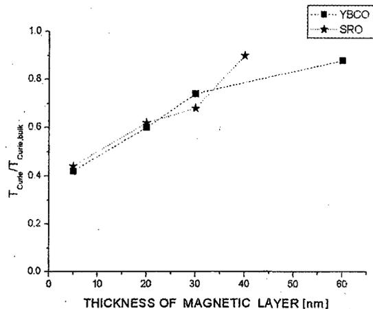
Fig. 5 Evolution of the Curie temperature for YBCO based superlattices with  $t_{\text{YBCO}} = 20\text{nm}$ .
