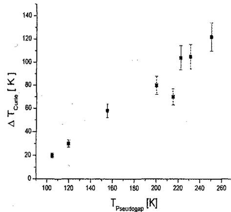
Fig. 8. Relation of the  $T_{Curie}$  reduction and the pseudogap temperature in symmetric YBCO/LCMO superlattices.
