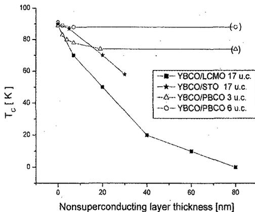
Fig.6 Comparison of  $T_C$  vs. thickness of non-superconducting layers in YBCO/LCMO, YBCO/SRO, and YBCO/PrBCO superlattices (explanations in the text).
