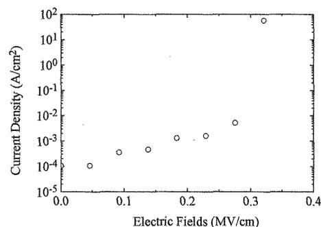
Fig.5 : I-V characteristic of  $\text{Cr}_2\text{O}_3$  thin film with 22 nm thickness. The size of measurement electrode was 0.45 mm  $\phi$ .
