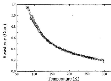
Fig.7 : Temperature dependence of resistivity of 50 nm thick YBCO film after  $\text{Cr}_2\text{O}_3$  deposition and annealing.
