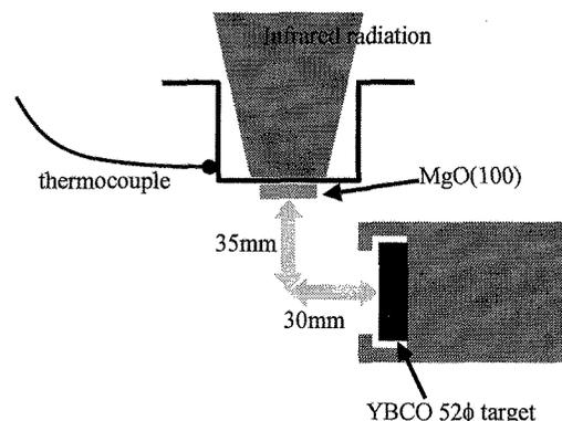
Fig.4 : Growth chamber of DC-RF magnetron sputtering for  $\text{YBa}_2\text{Cu}_3\text{O}_x$  thin films
