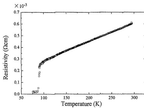
Fig.9 : Temperature dependence of resistivity of 200 nm thick YBCO film after Cr<sub>2</sub>O<sub>3</sub> deposition without annealing.
