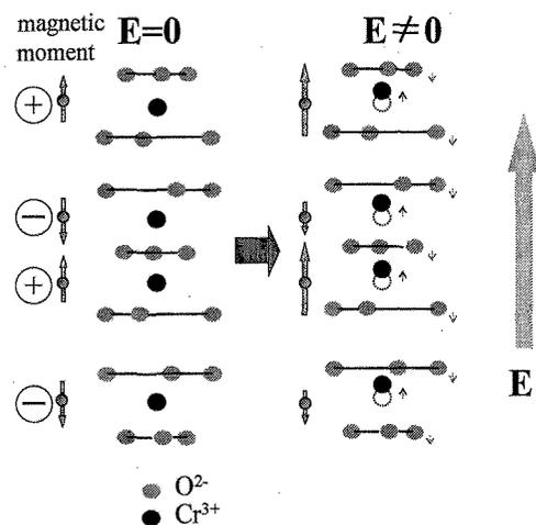
Fig.1 : Electric field effect of  $\text{Cr}_2\text{O}_3$
