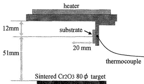
Fig.3 : Growth chamber of RF magnetron sputtering for  $\text{Cr}_2\text{O}_3$  thin films
