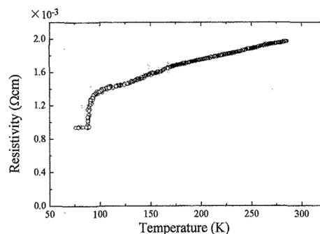
Fig.8 : Temperature dependence of resistivity of 200 nm thick YBCO film after  $\text{Cr}_2\text{O}_3$  deposition and annealing.
