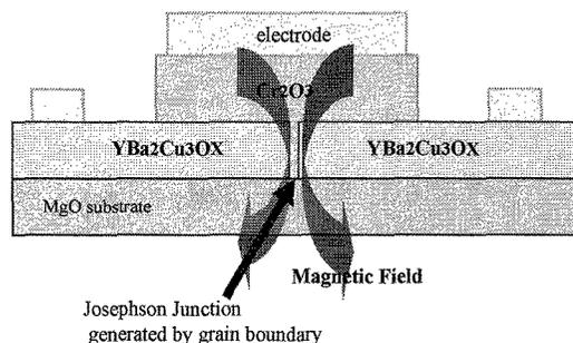
Fig.2 : Schematic image of Josephson magnetolectric field effect transistor (JMEET)
