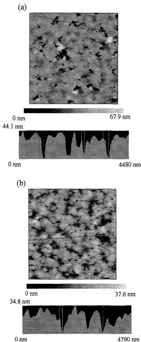
Fig.6 :  $5\mu\text{m}^2$  AFM images and line profiles of (a) 50 nm thick YBCO and (b) 200 nm thick YBCO films.
