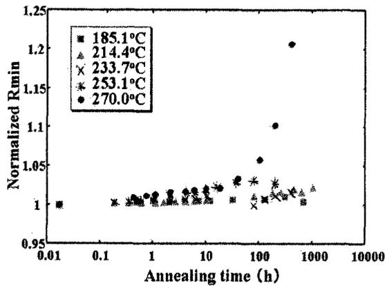
Fig.2. Annealing time dependence of the normalized resistance for various annealing temperatures.
