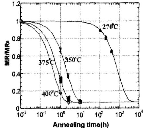
Fig.3. Annealing time dependence of the normalized MR ratio for temperatures greater than  $270^\circ\text{C}$ . The MR ratio is normalized against the saturation value of the MR ratio shown in Fig. 1. The solid lines are results fitted by using Eq. (2).
