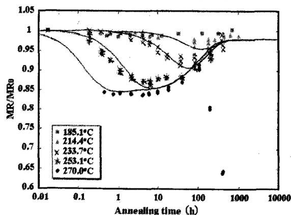
Fig.1. Annealing time dependence of the normalized MR ratio for various annealing temperatures. The solid lines are results fitted by using Eq. (1) in MTJs with the constant resistance
