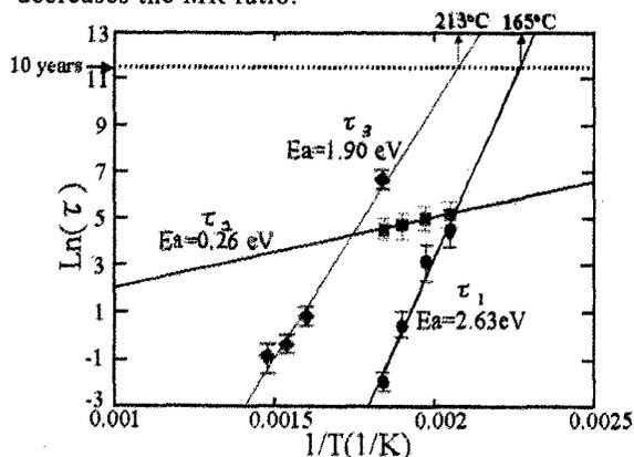
Fig.4. Annealing temperature dependence of the relaxation times  $\tau_1$ ,  $\tau_2$  and  $\tau_3$ . The solid lines are results fitted by using the equation  $\text{Ln}[\tau_i(T)] = E_{a_i}/k_B T - \text{Ln}[D_i]$ .
