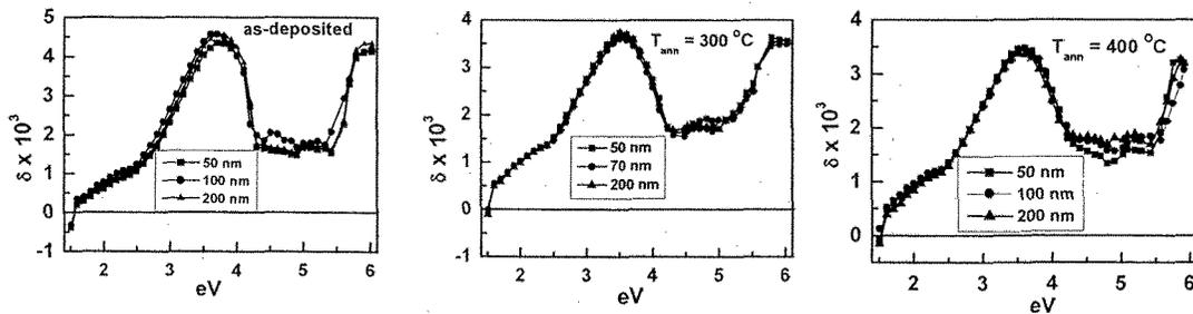
Fig. 6 Spectra of TKE obtained for the as-deposited and annealed Ni films.
