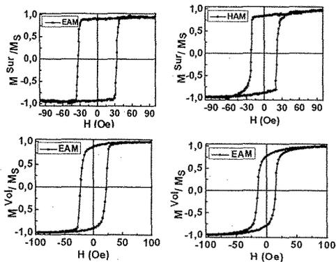
Fig. 1. Hysteresis loops, observed for the as-deposited Ni film of the 70-nm thickness at the in-plane magnetic field, applied parallel to the easy and hard axis of the magnetization ((EAM) and (HAM)), by the magneto-optical Kerr effect (MOKE) and vibrating sample magnetometer (VSM). The right panel shows AFM image of the film surface.
