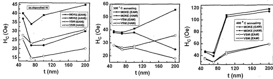
Fig. 4. The dependencies of the near-surface (MOKE) and volume (VSM) magnitudes of the coercivity along the easy and hard axes of the magnetization on the Ni film thickness.
