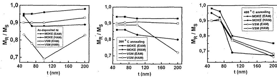
Fig. 5. The dependencies of the near-surface (MOKE) and volume (VSM) magnitudes of the remanent magnetization along the easy and hard axes of the magnetization (EAM and HAM) on the Ni film thickness.
