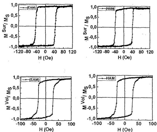
Fig. 3. Hysteresis loops, observed by MOKE and VSM for the annealed at  $T=400^{\circ}\text{C}$  Ni film of the 70-nm thickness at the in-plane magnetic field, applied parallel to EAM and HAM. The right panel shows AFM image of the film surface.
