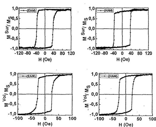
Fig. 2. Hysteresis loops, observed by MOKE and VSM for the annealed at  $T=300^{\circ}\text{C}$  Ni film of the 70-nm thickness at the in-plane magnetic field, applied parallel to EAM and HAM. The right panel shows AFM image of the film surface.
