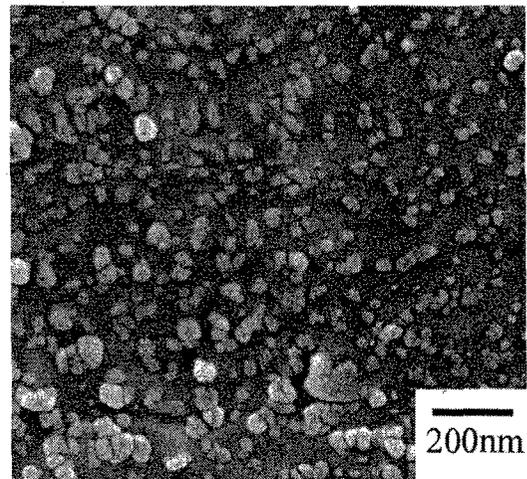
Fig.2 Microstructure of the powder (Cu: 0.5mass%).
