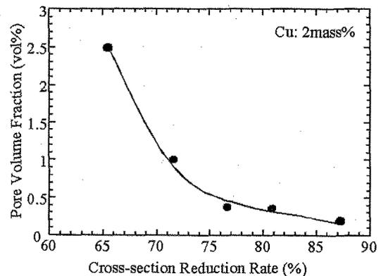
Fig. 3 Relation between pore volume fraction and cross-section reduction rate.
