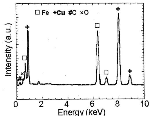
Fig. 6 EDS from a precipitate observed by TEM.
