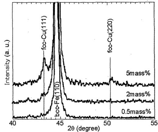
Fig.1 X-ray diffraction pattern of the powder.
