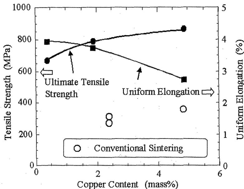
Fig. 7 Plots of ultimate tensile strength and uniform elongation of the consolidated samples against copper content.
