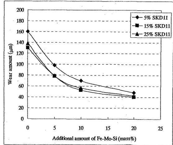
Fig.7 Relationship between wear amount and amount of hard particles
