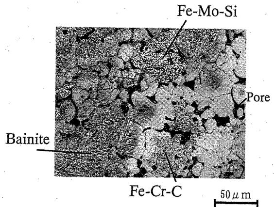
Photo 1 Microstructure of developed VSI
