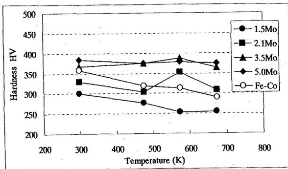
**Fig.2 Relationship between high temperature hardness and amount of molybdenum**
