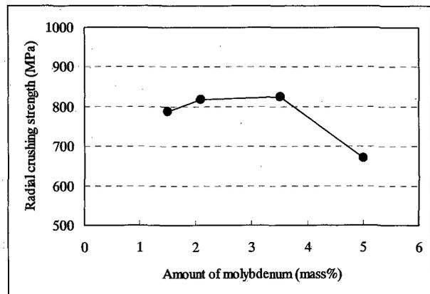
**Fig.3 Relationship between radial crushing strength and amount of molybdenum**
