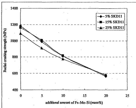
Fig.8 Relationship between radial crushing strength and amount of hard particles
