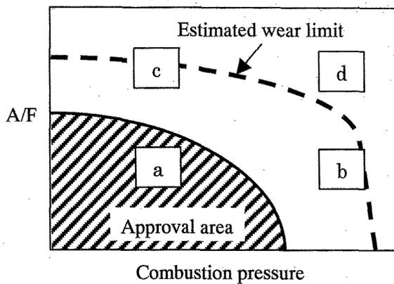
Fig.9 Diagram of condition of engine tests
