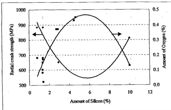
**Fig.4 Relationship between radial crushing strength and the amount of Silicon, Oxygen**
