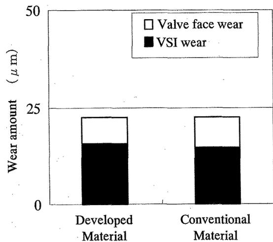
Fig.10 Results of actual engine test
