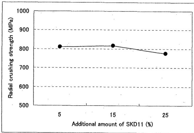
Fig.6 Relationship between radial crushing strength and the additional amount of Fe-Cr-C (SKD11)
