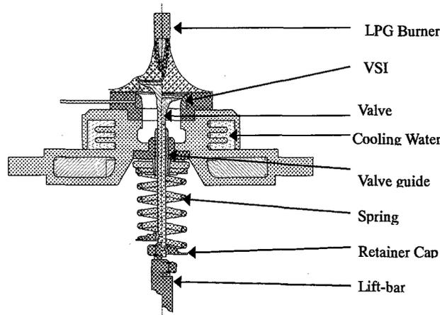
**Fig.1 VSI wear test apparatus**
