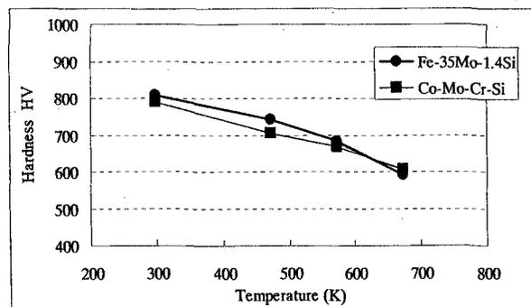
**Fig.5 High temperature hardness of Fe-Mo-Si and Co-Mo-Cr-Si**
