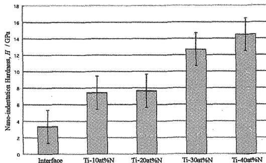
Fig. 6 the relation between nano-indentation hardness and composition of pure Ti to Ti-40at%N graded coating film.
