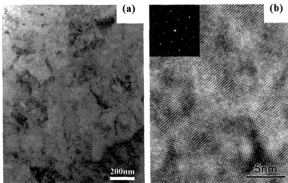
Fig. 5 TEM micrographs of TiN composite coating film. (a) TEM image. (b) HRTEM image and diffraction pattern of cubic TiN structure.
