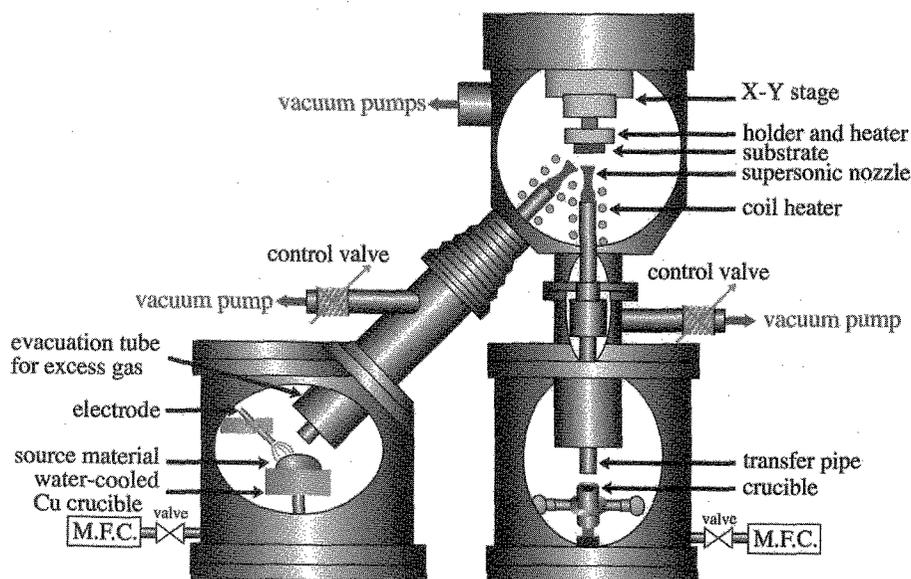
Fig. 1 Schematic diagram of Supersonic Free-Jet PVD apparatus.
