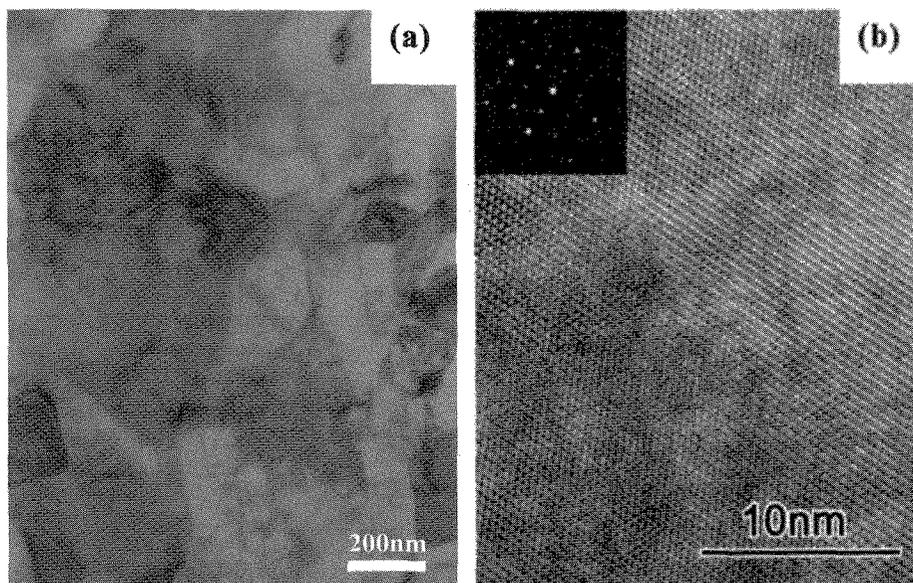
Fig. 3 TEM micrographs of Ti-Al composite coating film. (a) TEM image. (b) HRTEM image and diffraction pattern of  $D0_{22}$  structure.
