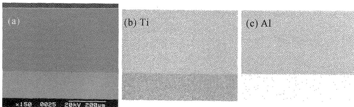
Fig. 2 SEM image of Ti-Al composite coating on Ti substrate and the corresponding X-ray mappings of Al and Ti elements.
