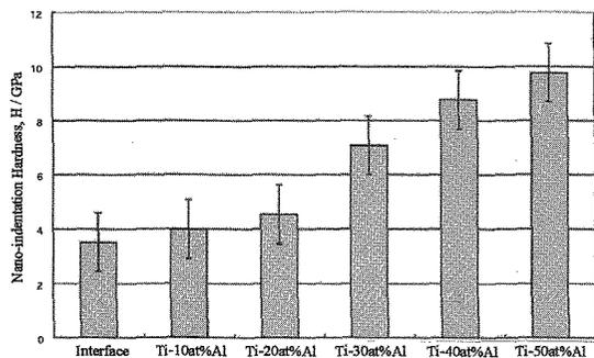
Fig. 4 the relation between nano-indentation hardness and composition of pure Ti to Ti-50at%Al graded coating film.
