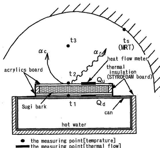
Figure 1 The simple calibration method: Measuring points of temperature and thermal flow of test piece
