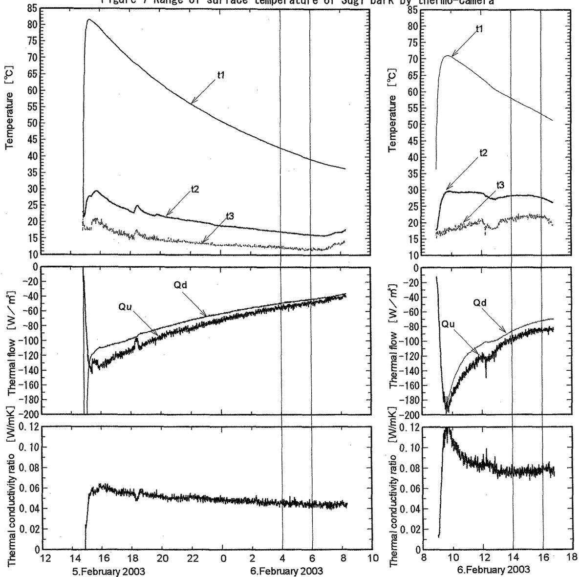
Figure 8 Fluctuation of temperature, thermal flow and thermal conductivity of STYROFOAM test piece
