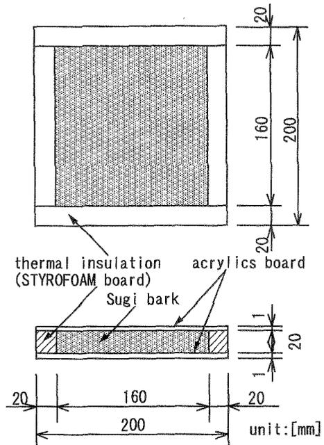
Figure 2 Size of test piece
