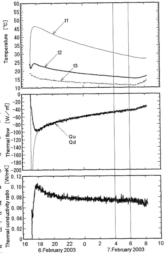
Figure 10 Fluctuation of temperature, thermal flow and thermal conductivity of Sugi bark (finely blended) test piece
