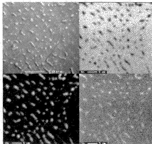
Fig. 3 SEM image and EPMA maps of Sn-3.5Ag-8In after reflow treatment.
