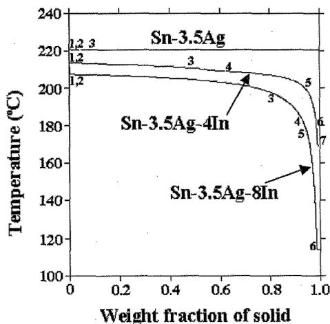
Fig. 5 Relationship between solid fraction-temperature by Scheil's calculation by ThermoCalc with Adamis7.
