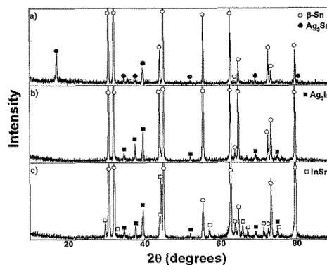
Fig. 2 XRD patterns from three alloys: (a) Sn-3.5Ag, (b) Sn-3.5Ag-4In, and (c) Sn-3.5Ag-8In.
