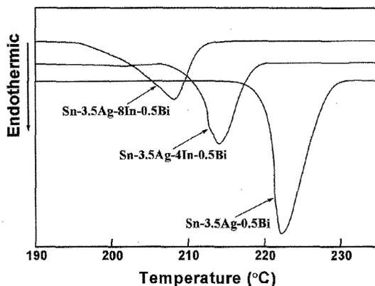
Fig. 4 DSC curves for the three solders on heating.
