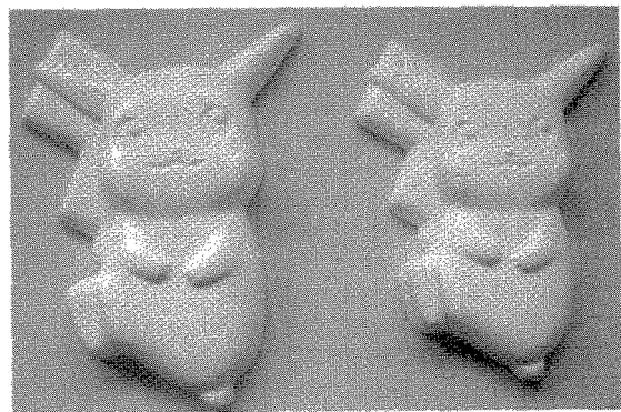
Fig. 6 Photograph of a green body (left) and a sintered body (right) fabricated by the proposed DCC method.
