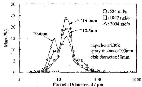
Fig. 4 The effects of disk rate and size on hybrid atomization.
