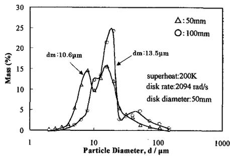
Fig. 5 The effect of spray distance on hybrid atomization.
