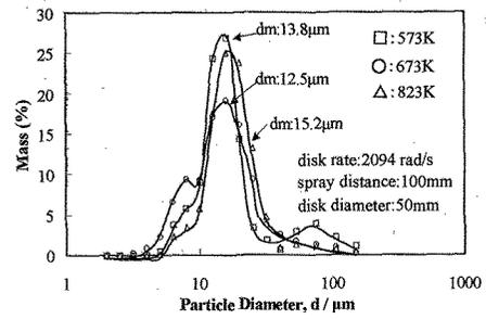
Fig. 3 The influence of superheat on hybrid atomization.
