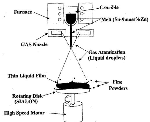
Fig. 1 A schematic diagram of the hybrid atomization procedure.
