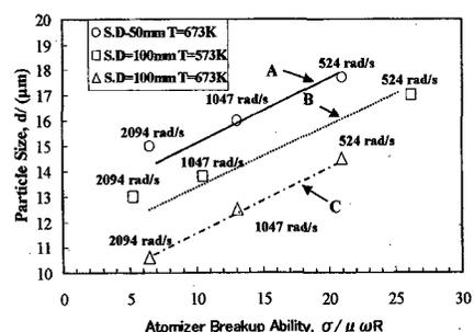
Fig. 6 The influence of delivery tube diameter on the particle size distribution.
