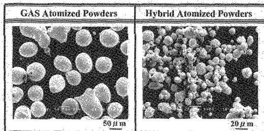
Fig. 2 SEM comparison of powders by hybrid atomization and gas atomization.
