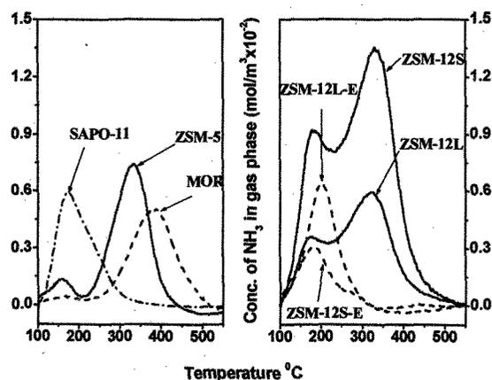
Fig. 2.  $NH_3$ -TPD profiles of zeolites
