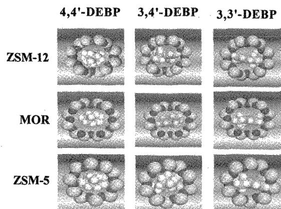
Fig. 6 The MG picture shows the fitting of DEBP isomers (CPK model) inside ZSM-12, MOR and ZSM-5 pores (cross-section of the 10 and 12-MR).
