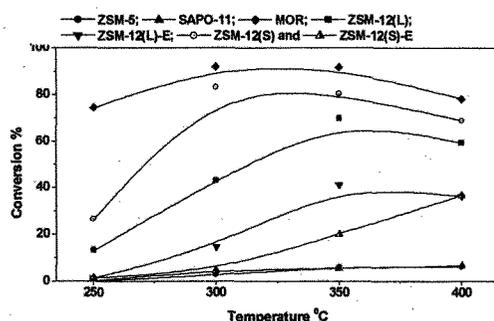
Fig. 3. Effects of reaction temperature on catalytic activity of zeolite. Reaction conditions: Feed=1:5:5.5 moles; BP: EtOH: Cy; WHSV = 1)
