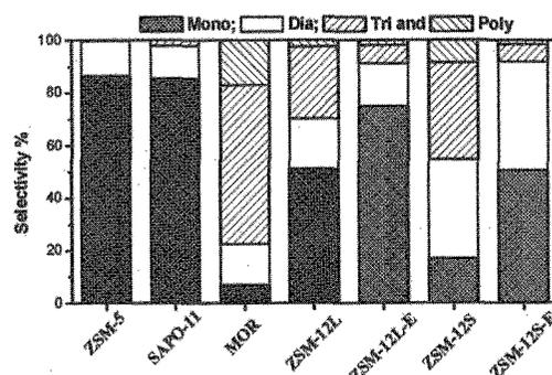
Fig. 5. Distribution of alkylated products over zeolites (Reaction conditions: temperature =300 °C and feed= 1:5:5.5 moles, BP: EtOH: Cy).
