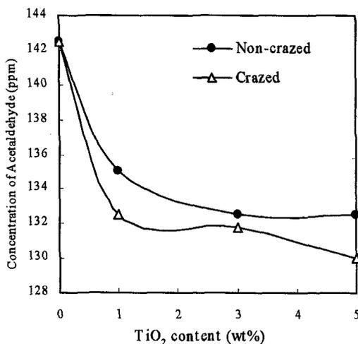
Fig. 8 Relation between concentration of acetaldehyde after 60 min and content of TiO<sub>2</sub>
