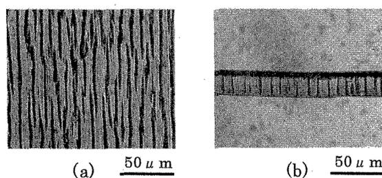
Fig.3 Optical micrographs of crazed film. (a) Surface, (b) cross-section.
