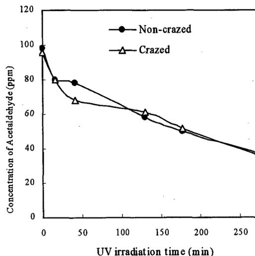
Fig.7 Relation between concentration of acetaldehyde and UV irradiation time for film with 5wt%  $\text{TiO}_2$ .
