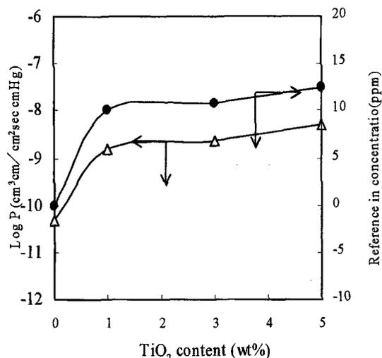
Fig. 10 Relation between permeability (N<sub>2</sub> gas) and difference in concentration of acetaldehyde for crazed film with TiO<sub>2</sub> of 5wt%.
