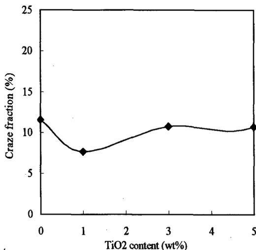
Fig.5 Craze fraction of crazed film with  $\text{TiO}_2$  content.
