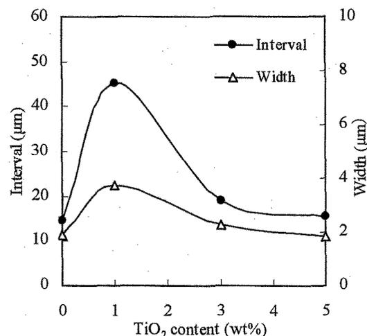
Fig.4 Width and interval of crazed film with  $\text{TiO}_2$  content.
