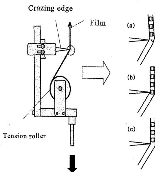
Fig.2 Schematic diagram of crazing device.
