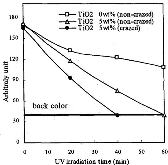
Fig.6 Color change of methylene blue by UV irradiation.
