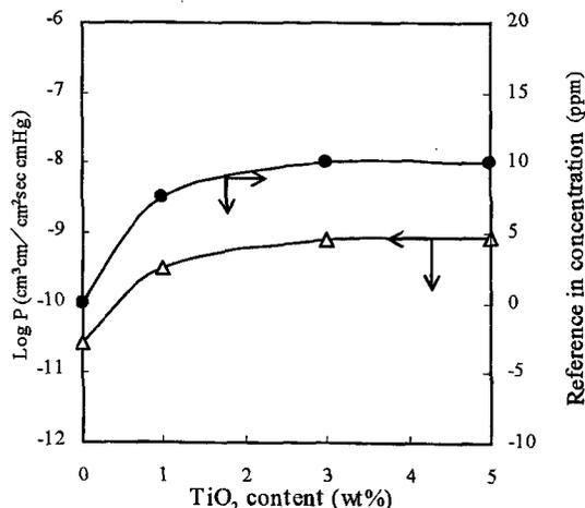
Fig. 9 Relation between permeability (N<sub>2</sub> gas) and difference in concentration of acetaldehyde for non-crazed film with TiO<sub>2</sub> of 5wt%.
