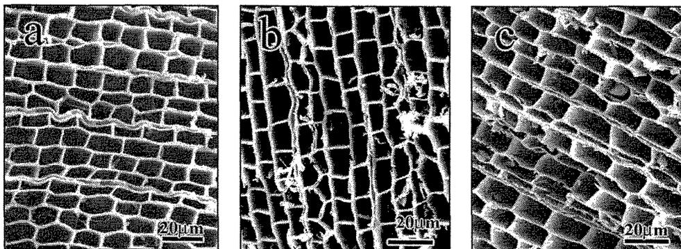
Fig. 7 SEM images of morph-genetic ceramic specimens
