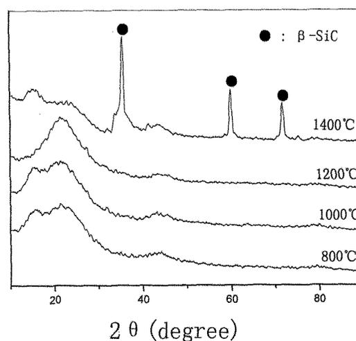
Fig. 2 XRD patterns of wood specimens sintered from 800 to 1400°C after infiltrating with silicone resin
