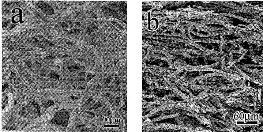
Fig. 8 SEM images of (a)  $\text{Al}_2\text{O}_3$  fibers and (b)  $\text{SnO}_2$  fibers derived from cotton fibers
