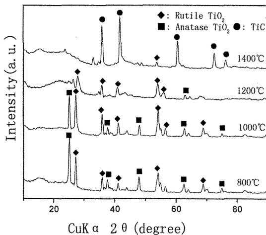
Fig. 6 XRD patterns of morph-genetic ceramics obtained at various temperatures after infiltration
