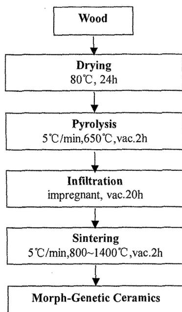
Fig. 1 Flow chart of the fabrication process
