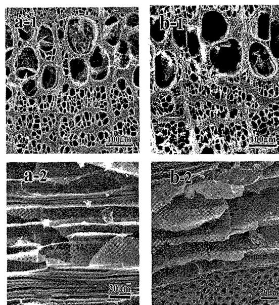
Fig. 3 SEM images of C-template and SiC/C (a: carbon preform; b: morph-genetic ceramics)
