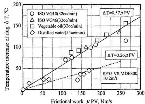
Fig.7 Relationship between temperature increase of ring and frictional work.
