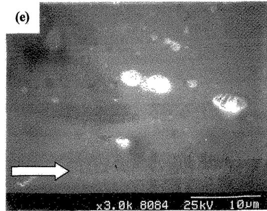
Fig.8 SEM micrographs of wear scars of woodceramics under water lubrication. (a); before friction, (b); after friction, (c); enlargement of (b), (d); X-ray analysis result of (c), (e); enlargement of smooth surface in (b). The white arrow indicates the frictional direction.
