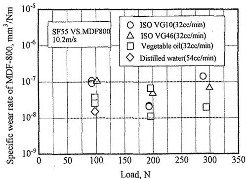
Fig.6 Relationship between specific wear rate of woodceramics and load.
