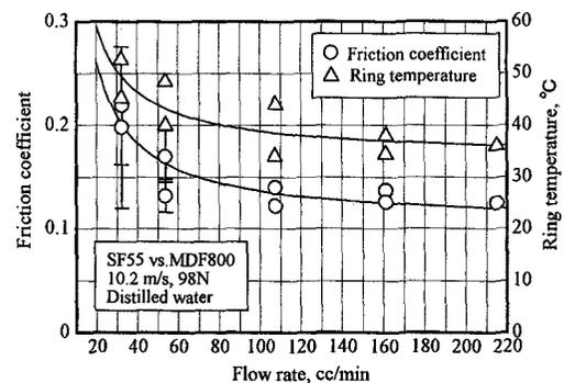
Fig.4 Effects of flow rate of distilled water on friction coefficient and ring temperature.
