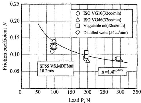
Fig.5 Relationship between friction coefficient and load.
