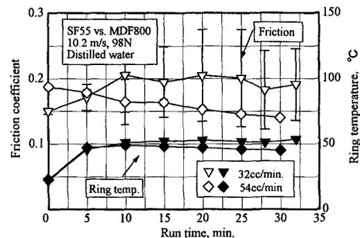
Fig.3 Friction and temperature curves under lubrication of distilled water.
