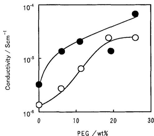
**Fig. 6** The ionic conductivity of the SPEs as a function of PEG content. (●): SPE made from POEM<sub>5</sub> (POEM content=48wt%), (○): SPE made from POEM<sub>9</sub> (POEM content=35wt%)
