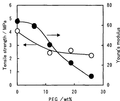
**Fig. 5** The tensile strength and Young's modulus of the SPEs using the POEM<sub>5</sub> graft copolymer as a function of PEG content (POEM content=48wt%).
