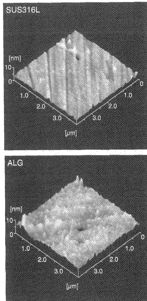
Fig. 2 AFM images of SUS316L and ALG surface
