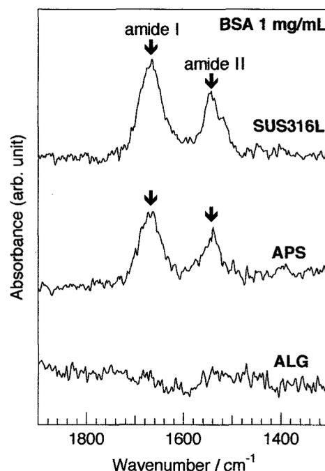
Fig. 4 FT-IRRAS spectra for BSA adsorbed on SUS316L, APS and ALG in a concentration of 1 mg/mL
