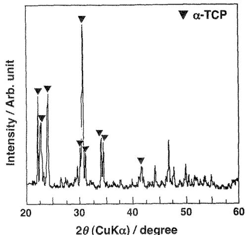
Fig 2 Powder X-ray diffraction pattern of the porous ceramics.
