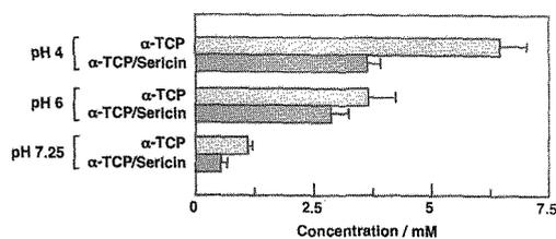
Fig. 6  $\text{Ca}^{2+}$  concentration of the buffer solutions at various pH after soaking of  $\alpha$ -TCP and  $\alpha$ -TCP/Sericin for 7 d (n=5).
