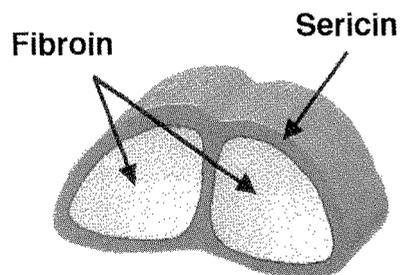
Fig. 1 Cross-sectional view of raw silk fiber.
