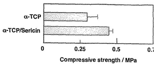
Fig. 4 Compressive strength of  $\alpha$ -TCP and  $\alpha$ -TCP/Sericin (n=5).
