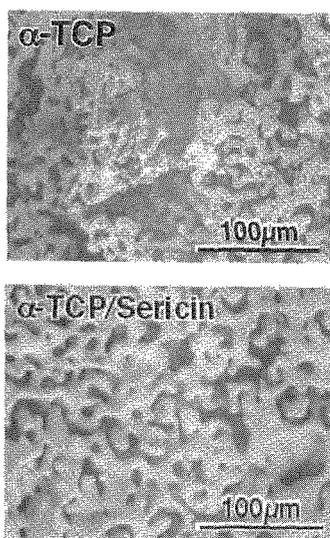
Fig. 5 SEM photographs of the inside of  $\alpha$ -TCP and  $\alpha$ -TCP/Sericin after soaking in buffer solution at pH 6 for 7 d.
