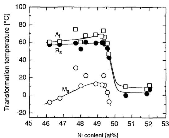
Fig. 2 The transformation temperatures of Ti-Ni films annealed at 600°C × 60 min → WQ as a function of Ni content in the films.
