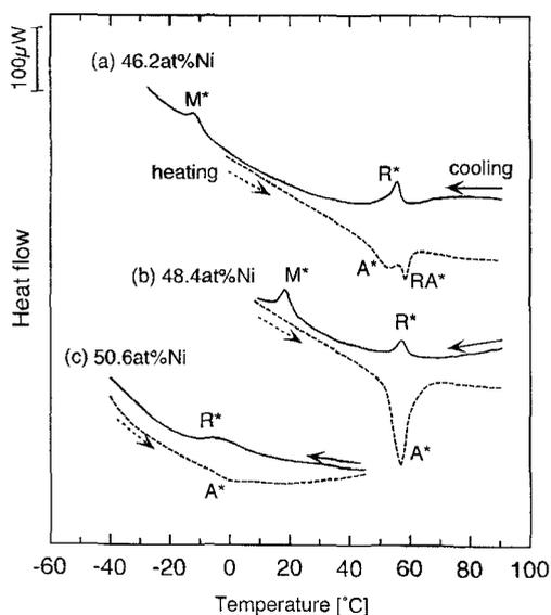
Fig. 1 Typical DSC curves of Ti-Ni films with various Ni contents annealed at 600°C for 60min followed by water quenching.
