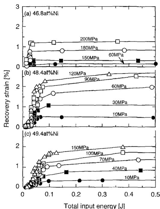
Fig. 4 The recovery strain under various applied stresses as a function of a total input energy.
