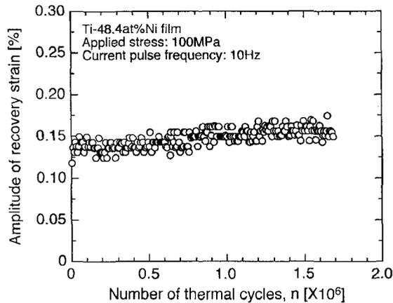
Fig. 6 The amplitude of recovery strain of Ti-48.4at%Ni film as a function of the number of thermal cycles.
