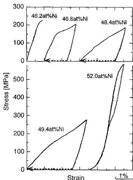
Fig. 3 Typical stress-strain curves of Ti-Ni films with various Ni contents. Dotted arrows indicate the recovery of the strain by Joule heat.
