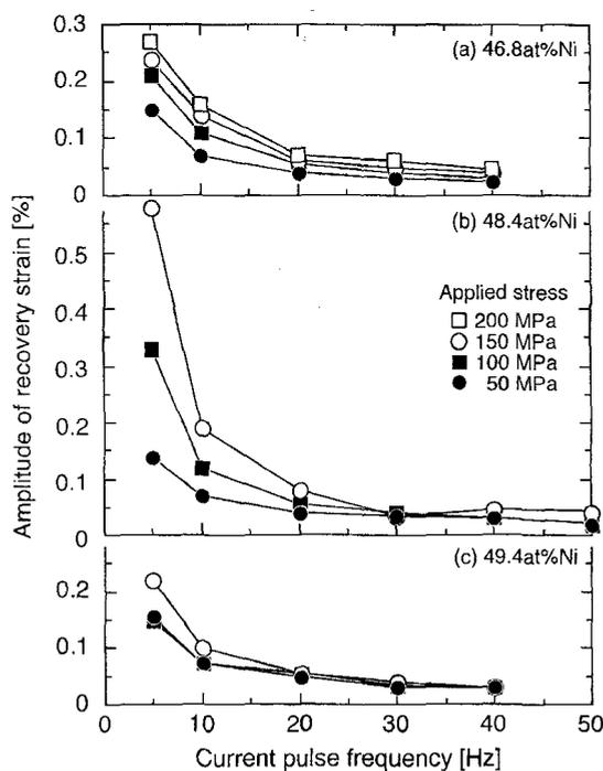
Fig. 5 The amplitude of the recovery strain found in the Ti-Ni films as a function of current pulse frequency.
