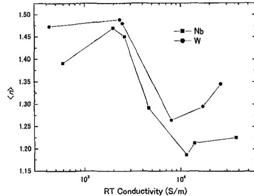
Fig.5 Average number  $\langle n \rangle$  of localized states in the intercluster conducting channels of Nb- and W-containing amorphous carbon-silicon nanocomposite films.
