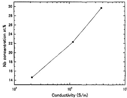
Fig.3 The dependence of RT conductivity of Nb containing film on metal concentration.
