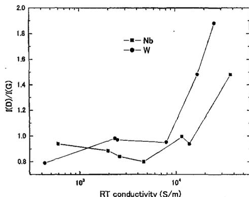
Fig.4 I(D)/I(G) peak ratio as a function of RT conductivity in metal-containing carbon-silicon nanocomposite films.
