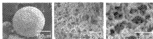
Fig.3 SEM photographs of the inorganic sample obtained from the Fe exchanged resin prepared by the method A (heat-treated at 1273K)
