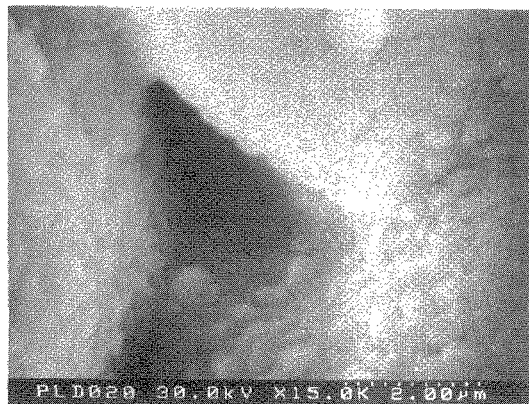
Fig.3 The FESEM image for the porous part of the LSGMCO thin film deposited at the substrate temperature of 800°C and the oxygen pressure of 133 Pa for 10min.
