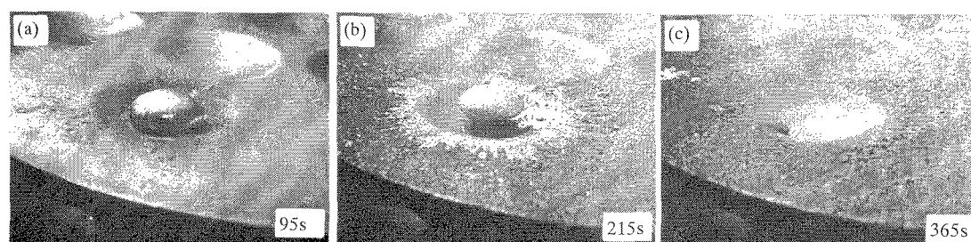
Fig.1 Disintegration phenomenon of Nb_{0.6}Zr_{0.25}Fe_{0.15} alloy in 0.1Mpa hydrogen pressure. (a) initial stage of disintegration (after 95 second in hydrogen ), (b) intermediate stage of disintegration (after 215 s ) and final stage ( after 365 s ).
