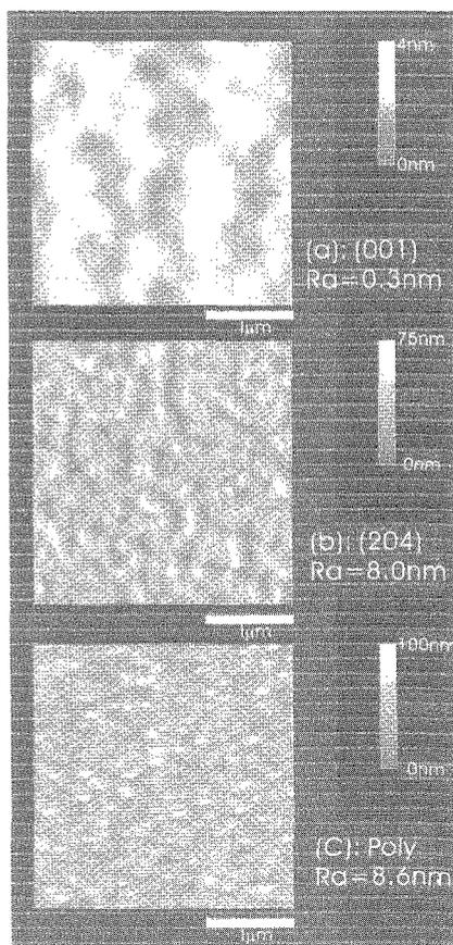
Fig.3. AFM micrographs of (a): anatase-(001), (b): anatase-(204), and (c): polycrystalline anatase, respectively.
