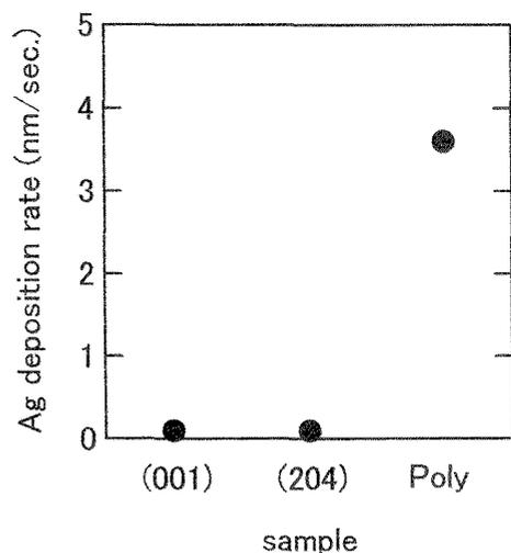
Fig.4. The photocatalytic activities of the films measured by photoreduction of Ag ions on the film surface (a): anatase-(001), (b): anatase-(204), and (c): polycrystalline anatase, respectively.
