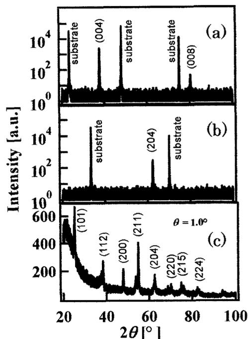
Fig.2. X-ray diffraction patterns of (a): anatase-(001), (b): Anatase-(204), and (c): polycrystalline anatase, respectively.
