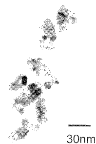
Fig. 1. TEM micrograph 3Y-TZP nanoaggregates.
