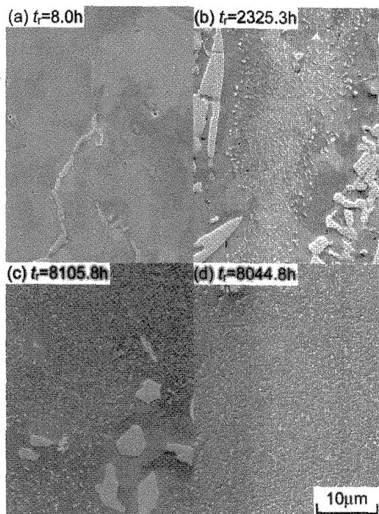
Fig. 2 SEM micrographs of the (a) base; (b) 6W-3Co; (c) 5C-3N and (d) 0C-7N steels creep ruptured at 923K and 120MPa. The  $t_r$  values indicated in each micrograph are times to rupture.
