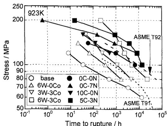
Fig. 1 Stress vs. time to rupture curves of the present studied steels and two conventional ferritic heat resistant steels using tempered martensitic microstructure.
