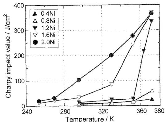
Fig. 6 Change in the Charpy impact values of the water quenched 5C-3N steels containing various contents of Ni with temperature.
