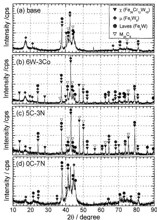
Fig. 3 X-ray diffraction profiles of the electrolytically extracted residue of (a) base; (b) 6W-3Co; (c) 0C-7N and (d) 5C-3N steels isothermally aged for 1000h at 923K.
