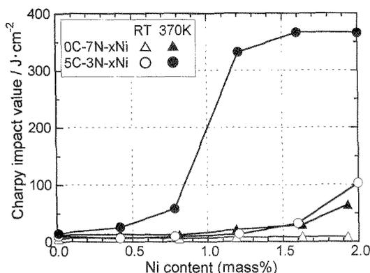
Fig. 5 Influence of Ni content on the Charpy impact values of the water quenched 0C-7N and 5C-3N steels at room temperature (RT) and 370K.
