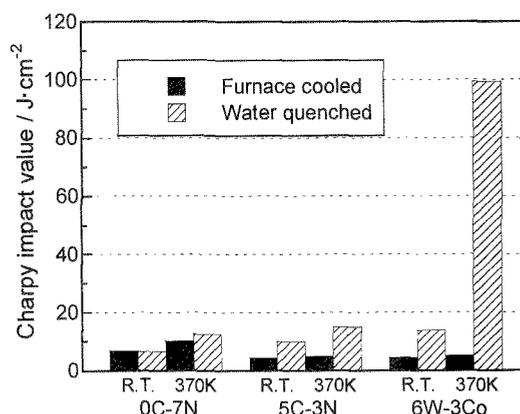
Fig. 4 Charpy impact values of the furnace cooled and water quenched 0C-7N; 5C-3N and 6W-3Co steels at room temperature (RT) and 370K.
