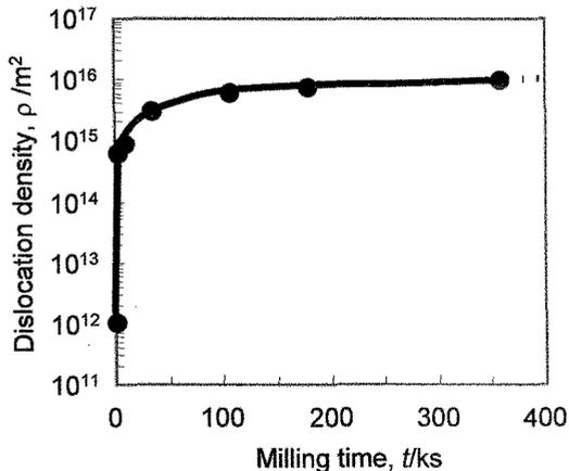
Fig. 5 Relation between MM time and dislocation density in the pure iron powder during MM treatment. The dislocation density is estimated from local strain shown in Fig.4.
