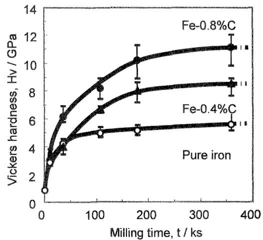
Fig. 8 Changes in hardness during MM treatment in Fe-C alloys with different carbon content.
