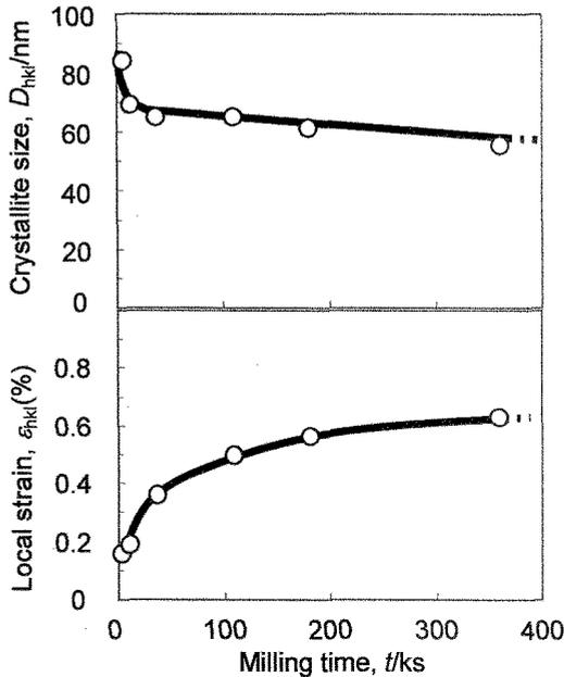
Fig. 4 Change in crystallite size and local strain in pure iron powder during MM treatment.
