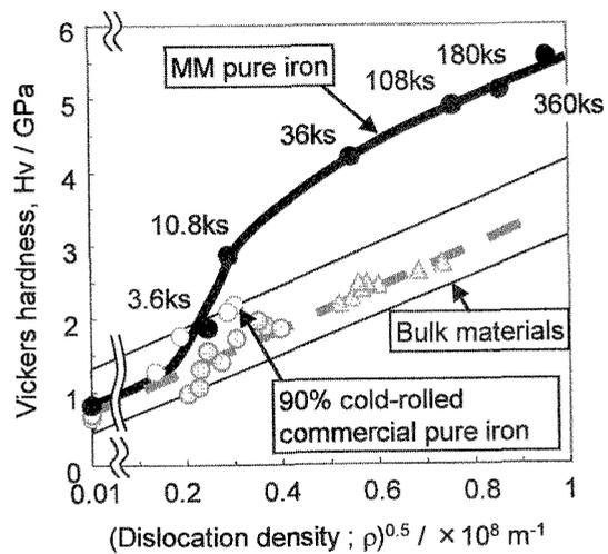
Fig. 6 Relation between hardness and square root of dislocation density;  $\rho^{0.5}$  in the pure iron powder (●)MM-treated for various times. MM time is shown in the figure and the data of bulk materials (Commercial pure iron;○, IF steel; △, and C free martensite; ▽) is also plotted in the figure.
