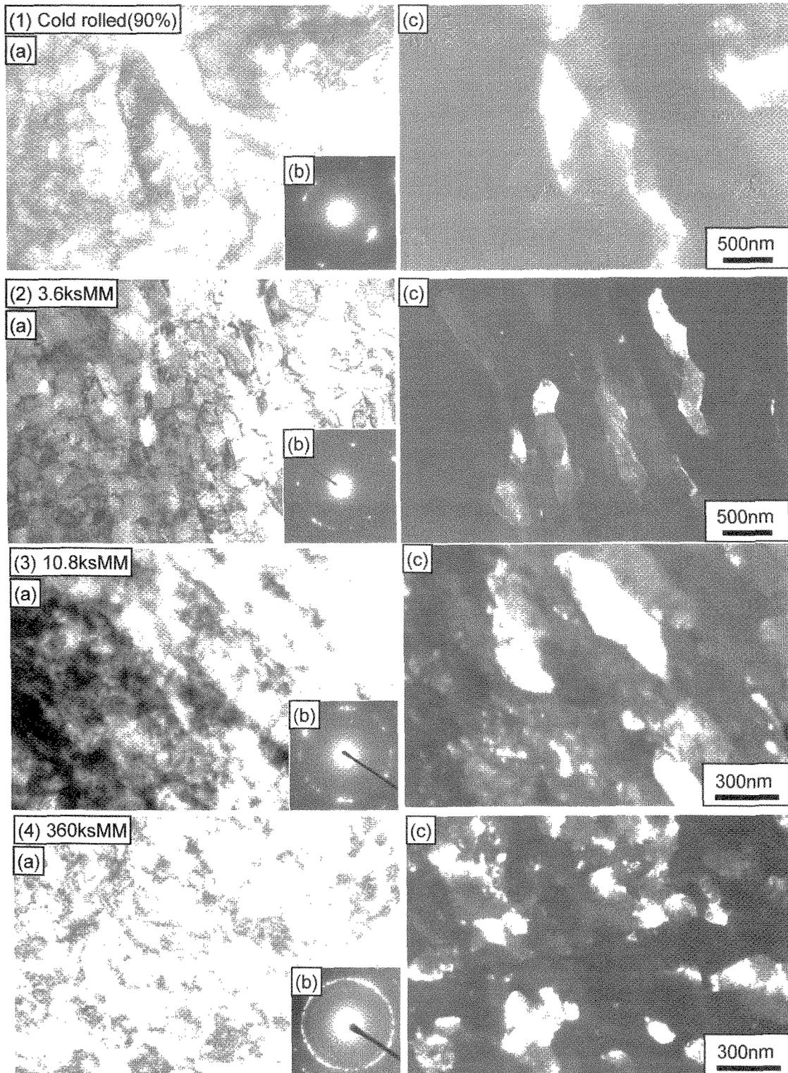
Fig. 7 TEM images of bulk pure iron cold-rolled by 90% (1) and pure iron powder MM-treated for various times; 3.6ks MM (2), 10.8ks MM (3) and 360ks MM (4) treatment. Bright field image (a), diffraction pattern taken from the area of  $1.5\mu\text{m}$  in diameter (b) and dark field image (c) from ferrite (110) diffraction spots.
