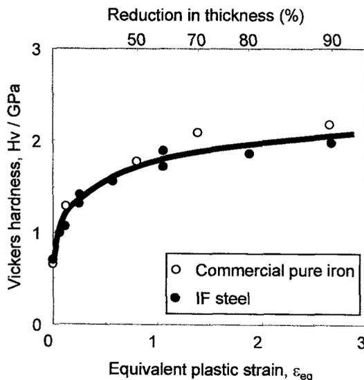
Fig. 1 Change of hardness in pure iron bulk sheet during cold rolling.
