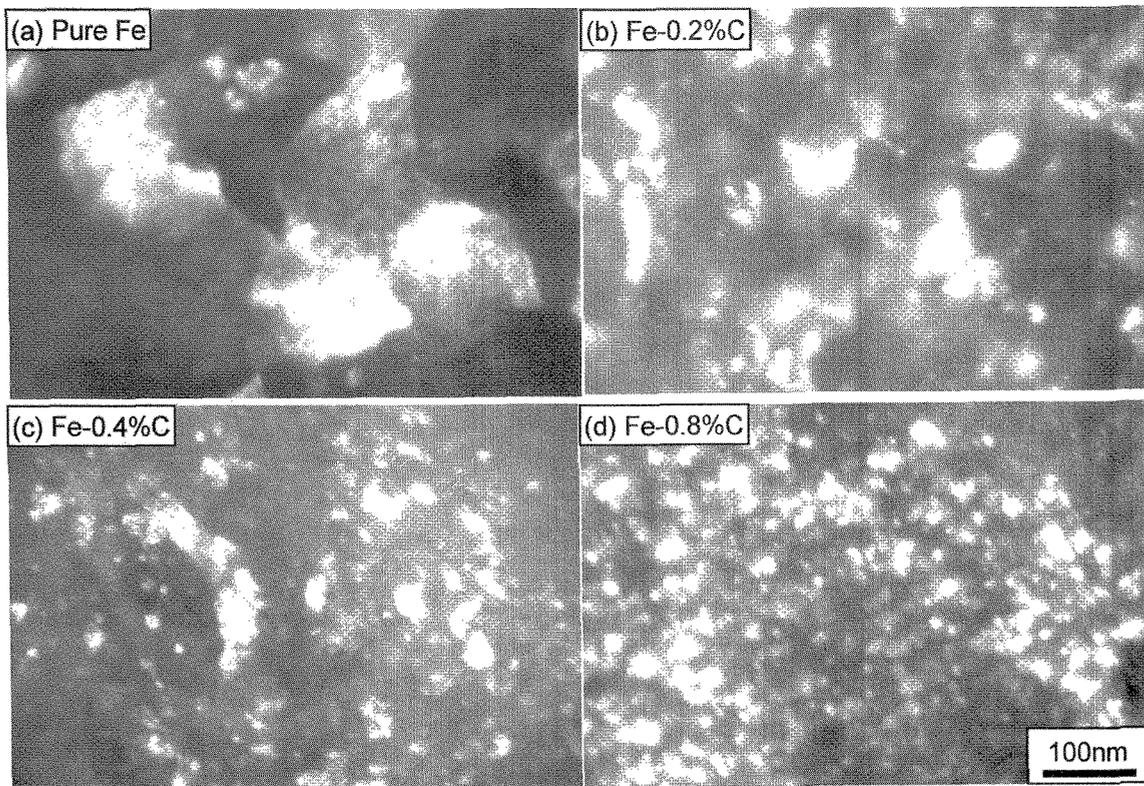
Fig. 9 Dark field images of Fe-C alloys MM-treated for 360ks; pure iron (a), Fe-0.2mass%C (b), Fe-0.4mass%C (c) and Fe-0.8mass%C (d).
