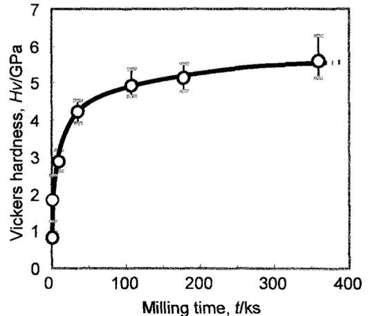
Fig. 3 Change in hardness of high purity iron powder during MM treatment.
