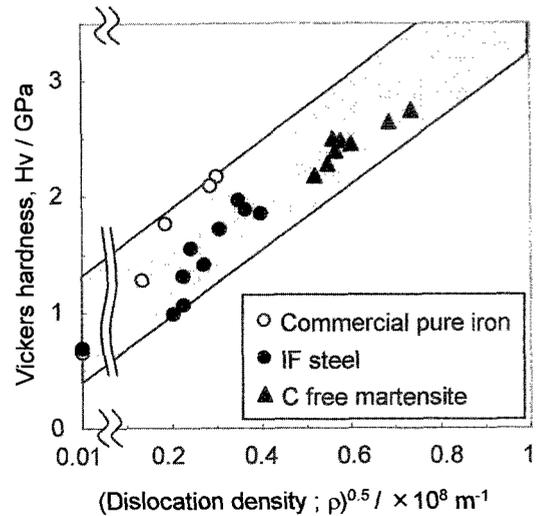
Fig. 2 Relation between hardness and square root of dislocation density;  $\rho^{0.5}$  in the pure iron sheet shown in fig.2. The data of carbon free martensite is also plotted in the figure for references.
