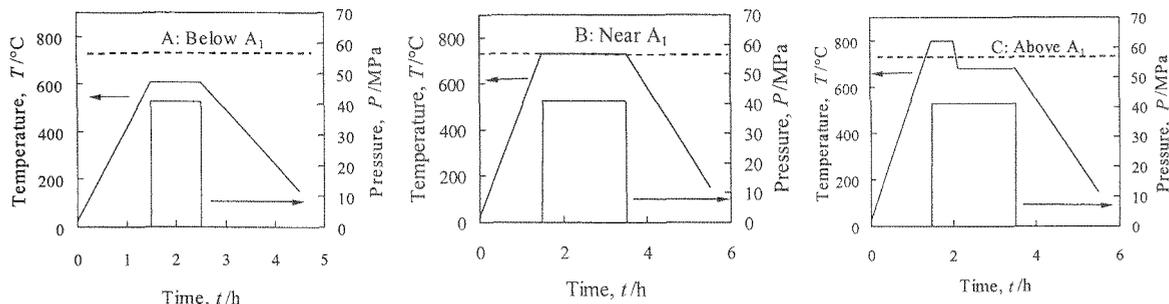
Figure 1 Various conditions of HP diagrams. A: Below  $A_1$  (610°C), B: Near  $A_1$  (730°C) and C: Above  $A_1$  (800°C)
