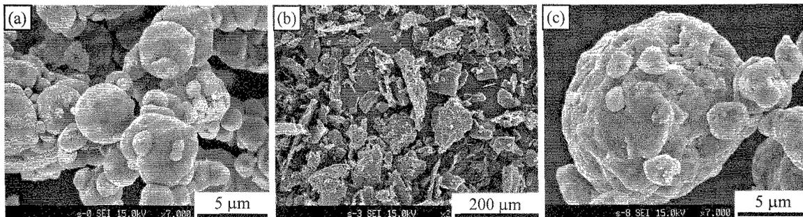
Figure 2 SEM images of as-received (a) iron and (b) graphite powders and (c) Fe-0.6C powders mixtures MAed for 300 h.
