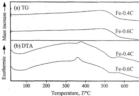
Figure 5 DTA-TG curves of Fe-0.4C and Fe-0.6C powders MAed for 200 h.
