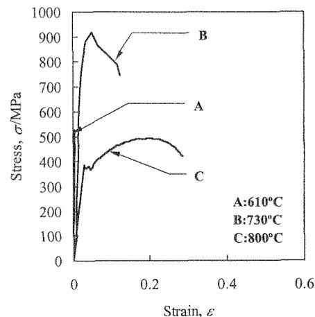
Figure 7 Stress-strain curves of tensile test for Fe-0.4C HPed compacts.
