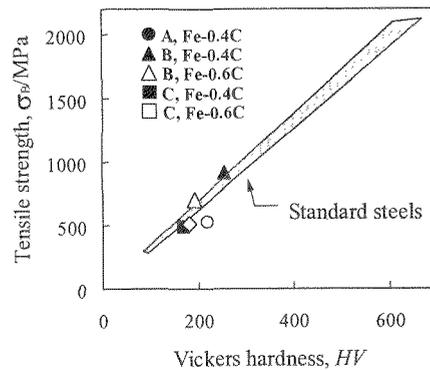
Figure 10 Relationship between tensile strength and Vickers hardness of the HPed compacts
