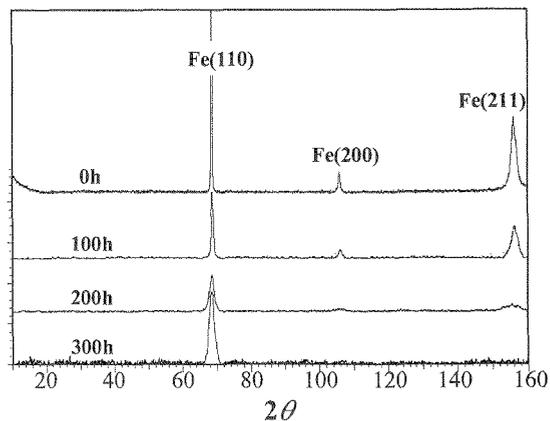
Figure 3 XRD patterns of Fe-0.6C powders MAed for various time.
