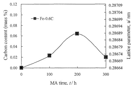
Figure 4 Changes in carbon content and iron lattice parameter as a function of MA time.
