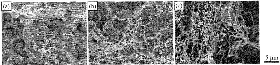
Figure 8 SEM images of the cross section of the fracture surface of the Fe-0.4C compacts HPed at (a) 610, (b) 730 and (c) 800°C after tensile test.
