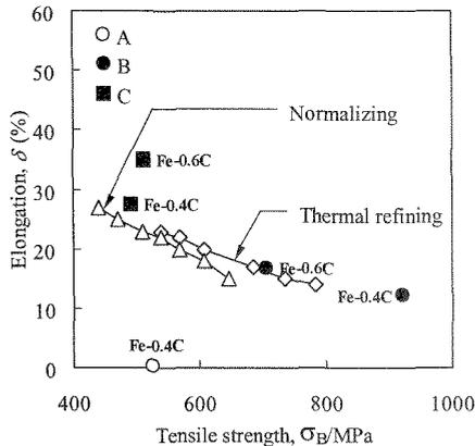
Figure 9 Relationship between tensile strength and elongation of the HPed compacts.
