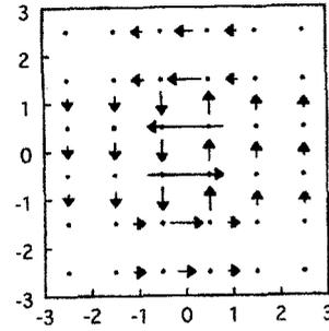
Fig 3 Stable core structure shown by Vitek's representation for non-linear potential with parameter  $\lambda=1.0$  in Eq.(1).
