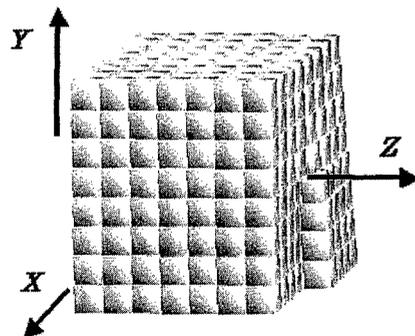
Fig. 1 Screw dislocation lying parallel to the  $z$  direction in a cubic lattice.
