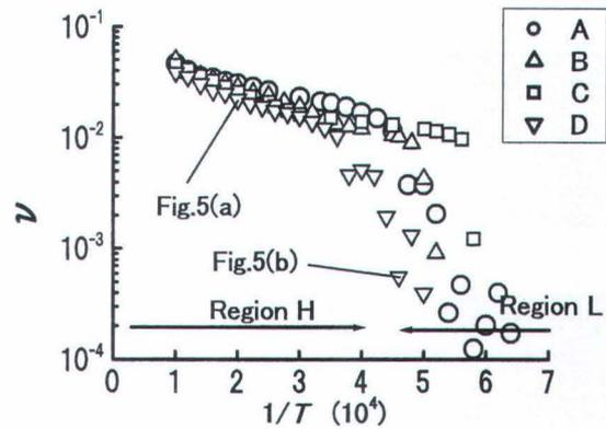
Fig. 4 Temperature dependence of frequency of thermally activated motions simulated from four different initial velocity distributions from A to D. The points marked by Fig.5(a) and (b) are detailed in Figs. 5.
