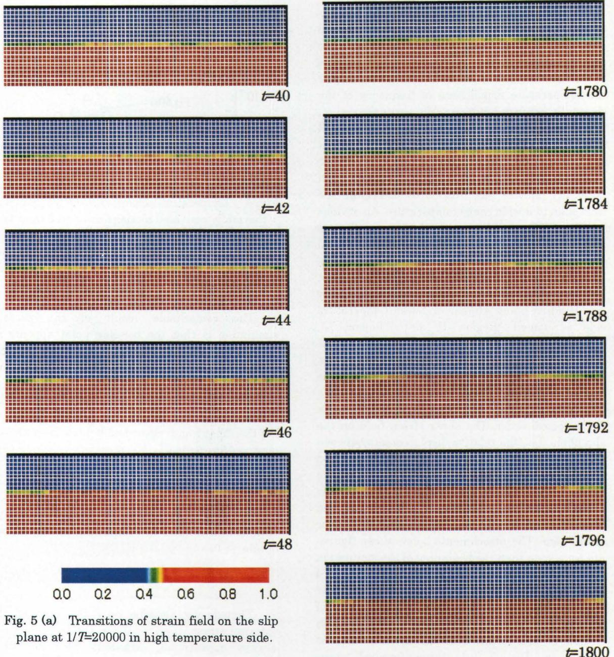
Fig. 5 (a) Transitions of strain field on the slip plane at  $1/T=20000$  in high temperature side.
