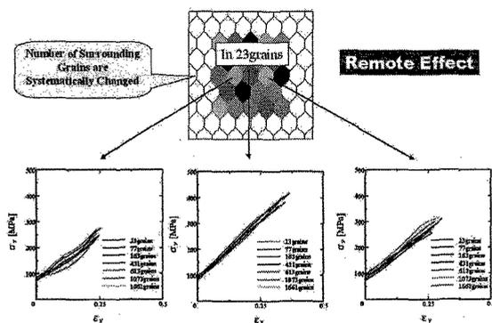
Fig. 8 Stress-strain responses of representative grains affected by number of surrounding grains implying "remote effect."
