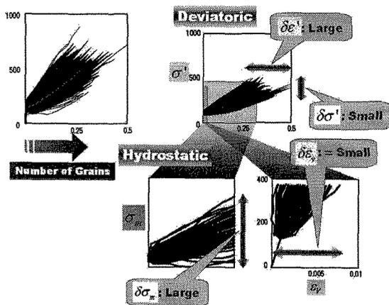
Fig. 6 Summary of simulation results demonstrating clear collective effects of increasing number of grains on stress-strain response of polycrystalline aggregate.
