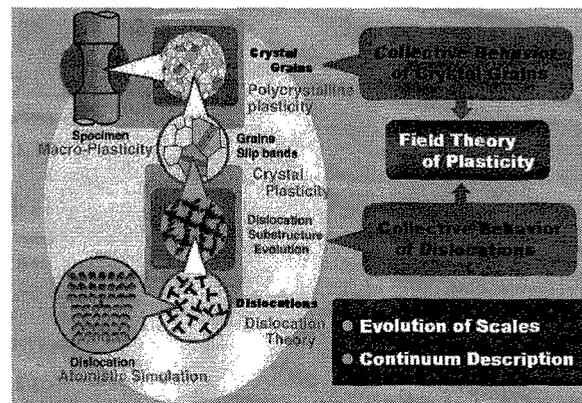
Fig. 1 Hierarchy of polycrystal plasticity and key scales for multi-scale modeling.
