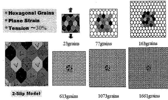
Fig. 3 Polycrystalline models used in FE analysis. Each grain is divided into several hundred to several ten meshes.
