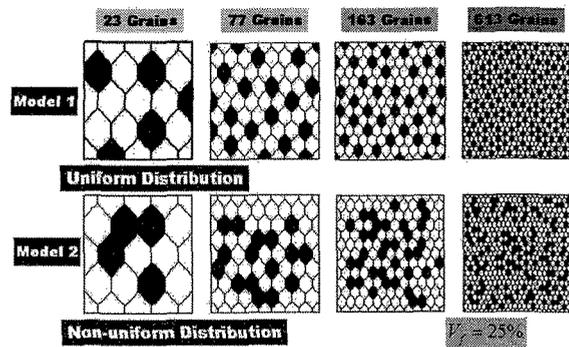
Fig. 11 Dual phase models used where hard grains having larger flow stress level are introduced with 25% volume fraction.
