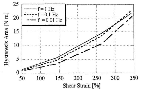
Fig.4 Energy dissipation (Second cycle of loading)
