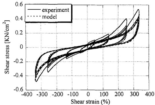
Fig.6b Stress-strain (f=1 Hz)
