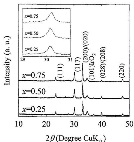
**Fig.6:** XRD profiles of 250 nm-thick BNT ( $x=0.25$ -0.75) polycrystalline thin films deposited on  $(101)\text{IrO}_2/\text{SiO}_2/\text{Si}$ .
