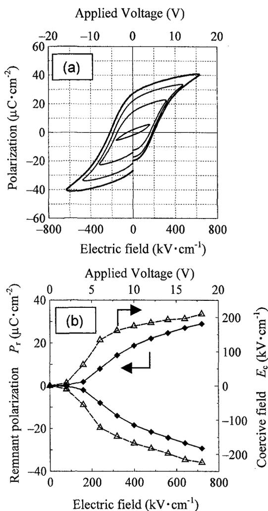
**Fig.4:** Room temperature ferroelectric properties in 250 nm-thick BNT thin film of  $x=0.25$  and  $T_{cr}=530$  °C. (a)  $P$ - $E$  hysteresis loops and (b) Saturated curves of  $P_r$  and  $E_c$ .
