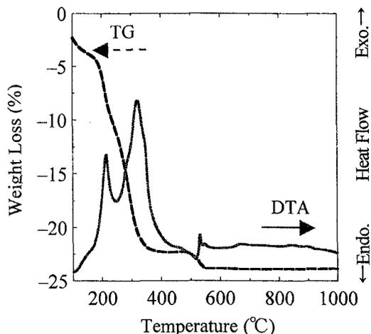
**Fig.1:** TG-DTA curves of BNT( $x=0.25$ ) powder.
