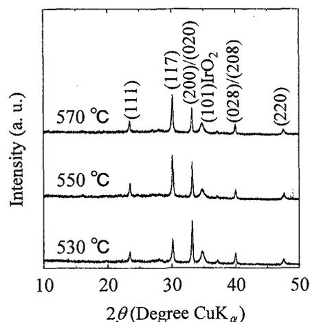
**Fig.2:** XRD profiles of  $\text{Bi}_{3.75}\text{Nd}_{0.25}\text{Ti}_3\text{O}_{12}$  ( $T_{\text{cr}} = 530$ – $570$   $^{\circ}\text{C}$ ) polycrystalline thin films deposited on  $(101)\text{IrO}_2/\text{SiO}_2/\text{Si}$ .
