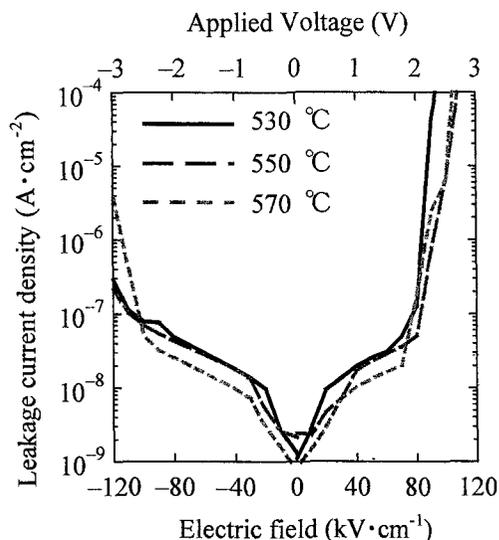
**Fig.3:** The room temperature leakage current density and electric field ( $J$ - $E$ ) characteristics in  $\text{Bi}_{3.75}\text{Nd}_{0.25}\text{Ti}_3\text{O}_{12}$  ( $T_{\text{cr}} = 530$ – $570$   $^{\circ}\text{C}$ ) polycrystalline thin films with the thickness of 250 nm.
