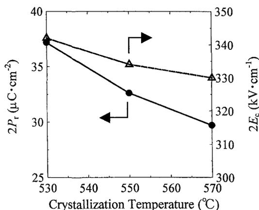
**Fig.5:** The  $T_{cr}$  dependence of measured  $2P_r$  and  $2E_c$  under the electric field of 400 kV/cm (10 V) at 50 Hz in 250 nm-thick BNT( $x=0.25$ ) films.
