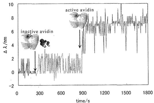
Fig. 9 Changes in  $\Delta\lambda$  of biotin tip induced by adding inactive and active avidin ( $1.0 \times 10^{-6}$ M).
