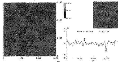
Fig. 8 AFM images of surface of biotin tip after soaking in avidin solution ( $1.0 \times 10^{-7}$ M pH=7.4).
