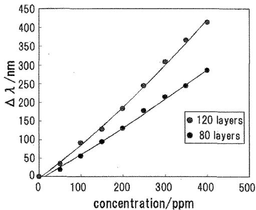
Fig.5 Changes in  $\Delta\lambda$  of polypeptide tip (80 and 120 layers) with various concentrations of *p*-*n*-butylphenol in water.
