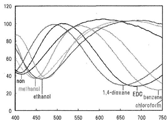
Fig. 3 Reflective VIS spectra of polypeptide tip (119 layers) with various vapor of organic solvents.
