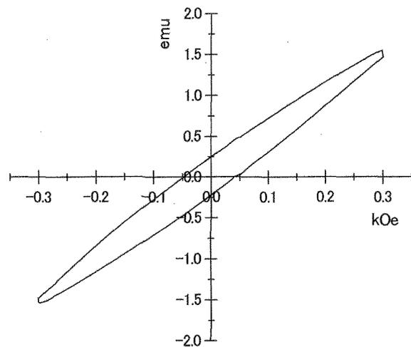
Fig.6 Magnetization curves under the magnetic field up to 300 Oe for the 30 vol% magnetite / 70 vol% hydroxyapatite composite prepared by hydrothermal method.
