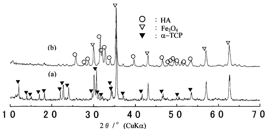
Fig.3 XRD patterns of (a) starting mixture of  $\alpha$ -TCP and  $\text{Fe}_3\text{O}_4$ , (b) the composite prepared by hydrothermal method. The sample (b) was first treated hydrothermally in the vapor of water at 120 °C for 10h, and secondly treated hydrothermally in the liquid phase at 200 °C for 10h.
