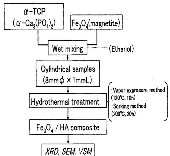
Fig.2 Preparation method of porous composites of magnetite / hydroxyapatite.
