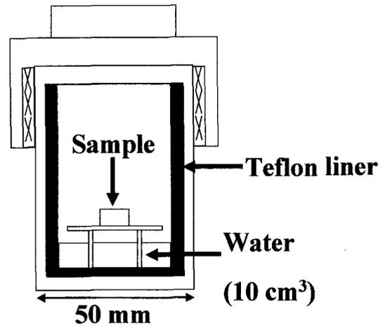
Fig.1 Schematic illustration of apparatus for hydrothermal treatment.
