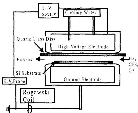
Fig. 1 Schematic diagram of DBD texturing system.
