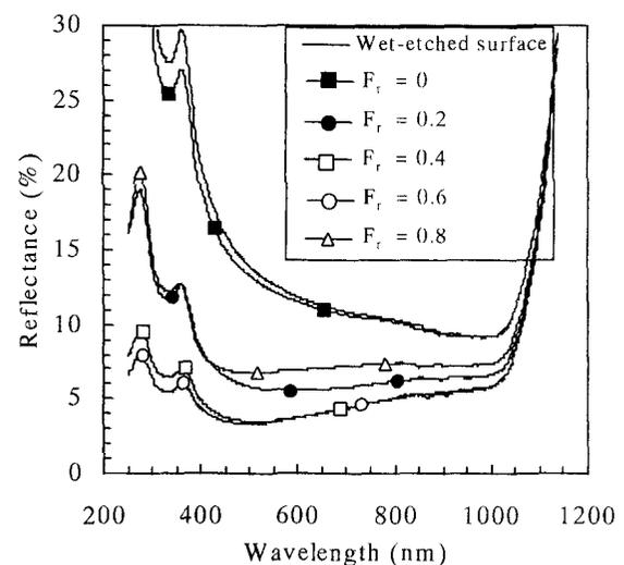
Fig. 3 Reflectance of the wet-etched surface and the DBD-treated surfaces at  $F_r=0, 0.2, 0.4, 0.6$  and 0.8.
