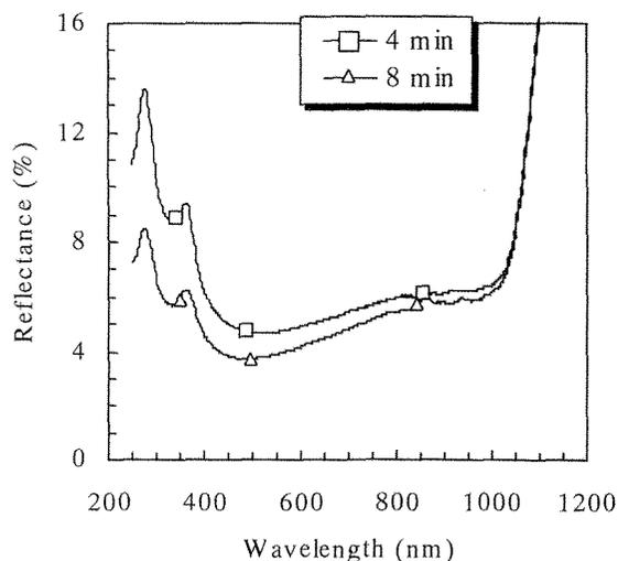
Fig. 7 Reflectance of the DBD-treated surfaces for 4 and 8 min when  $F_r = 0.4$ .
