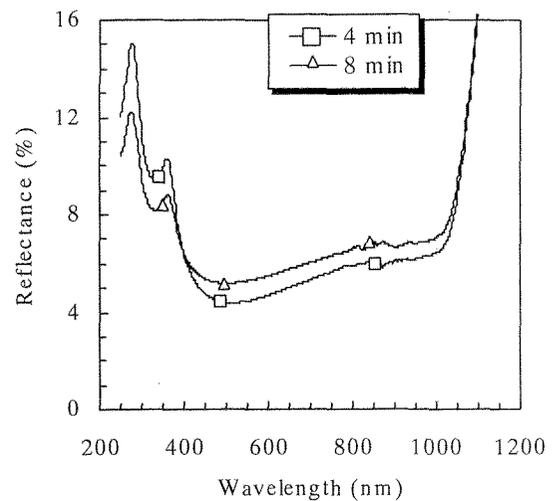
Fig. 5 Reflectance of the DBD-treated surfaces for 4 and 8 min when  $F_r=0.6$ .
