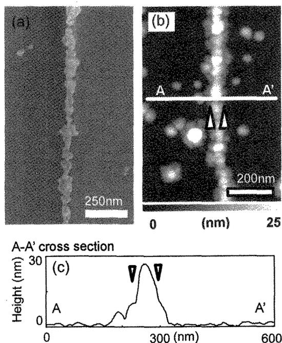
**Fig. 4.** (a) SEM images of a DNA- $2C_{16}N^+2C_1$  complex monolayer after silver electroless plating. The applied voltage was 1kV. (b) AFM images of wire-like structures fabricated using a platinum catalyst. (c) Cross-sectional profiles at A-A' in (b).
