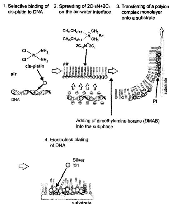
**Fig. 1.** A scheme for the nucleation of catalysts prepared from cis-platin and for fabricating nanowires along the template DNA molecules by electroless plating.
