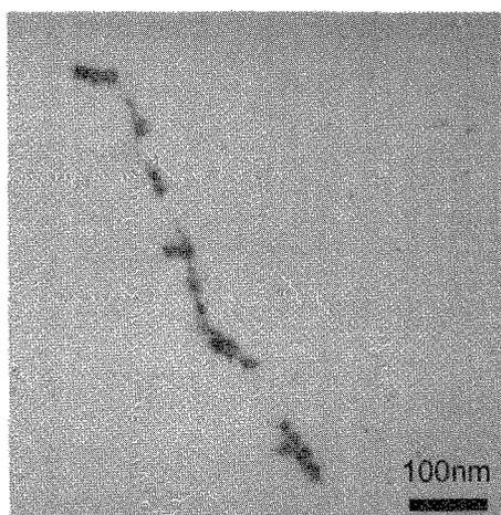
**Fig. 3.** TEM image of the polyion complex monolayer after reduction of cis-platin in a subphase by adding DMAB
