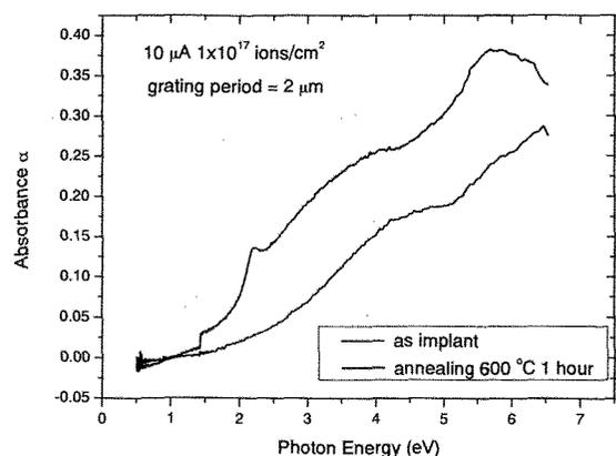
Fig. 4. Absorbance spectrum before and after annealing.
