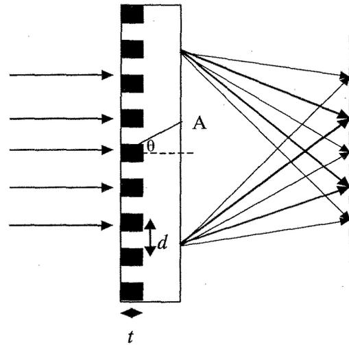
Fig. 7. Schematic of grating calculation.
