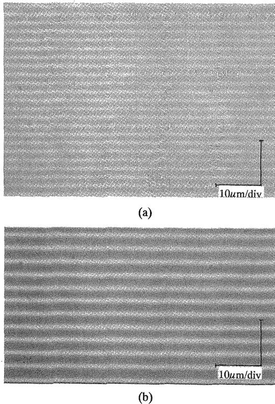
Fig. 1. Grating picture with different periodic parameter. (a) Periodic constant of  $2\ \mu\text{m}$  (b) Periodic constant of  $3\ \mu\text{m}$ .
