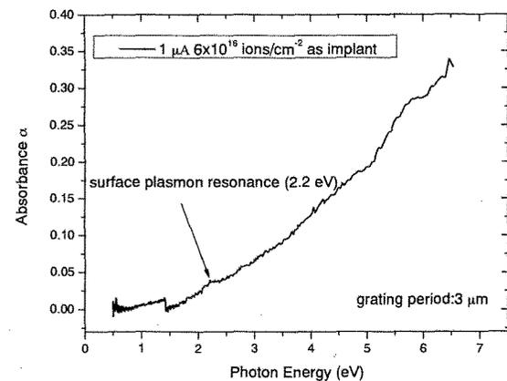
Fig. 3. Absorbance spectrum at  $1\ \mu\text{A}\ 6 \times 10^{16}$  ions/ $\text{cm}^2$ .
