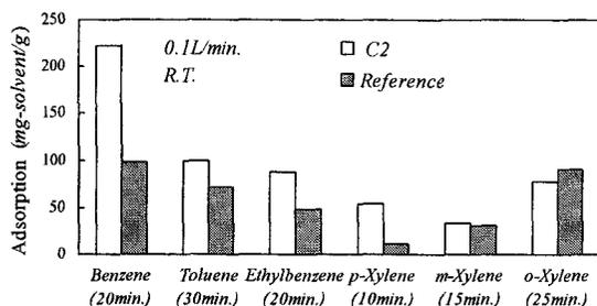
Fig. 5. Adsorption characters for several aromatic vapors by the reference and the specimen C2.
