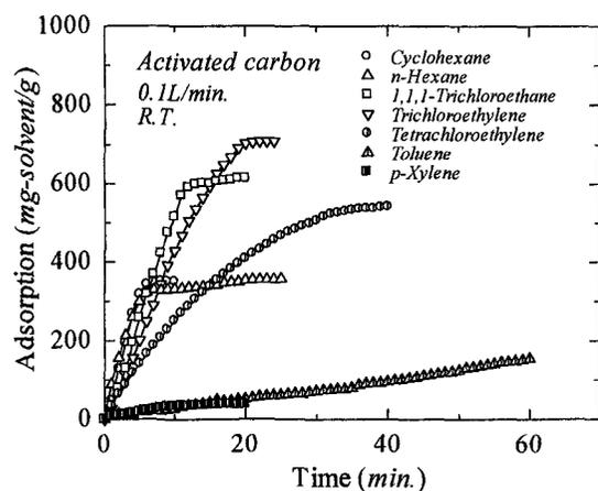
Fig.3. Adsorption of several organic solvents' vapors by the reference (activated carbon). (Extraction from Ref. [3])
