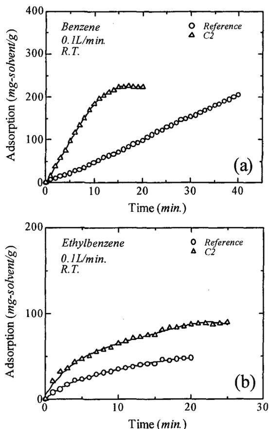
Fig.4. Adsorption of vapor of Benzene (a) and Ethylbenzene (b) by the reference and the specimen C2.
