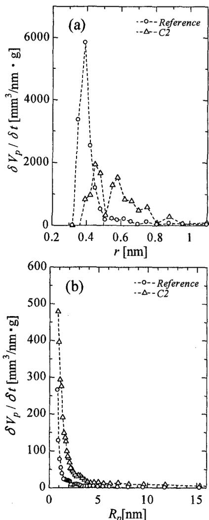
Fig.2. Pore size distributions of the reference and the specimen C2 calculated by MP (a) and Dollimore-Heal (b) method. (Extraction from Ref. [3])
