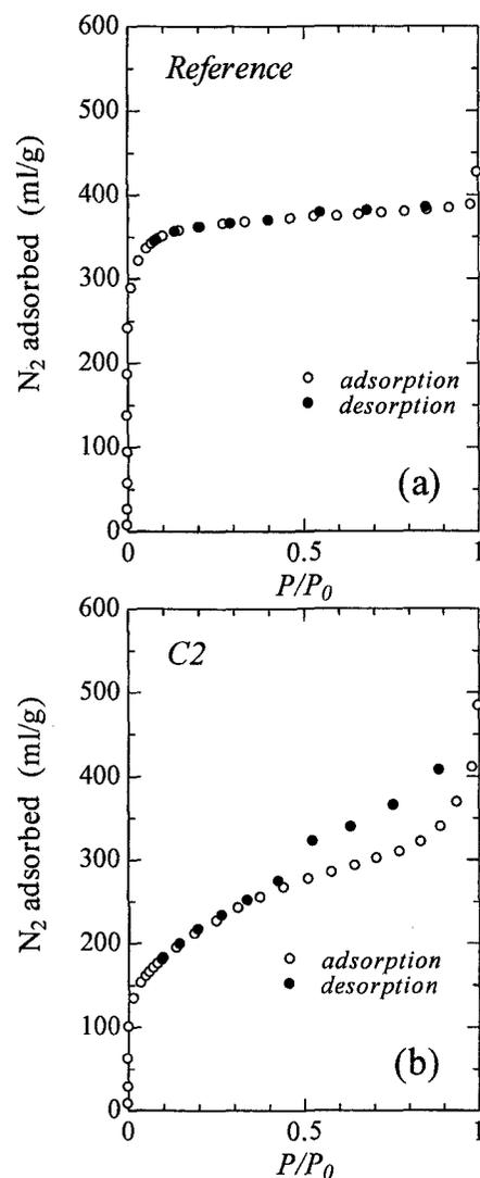
Fig.1.  $N_2$  adsorption and desorption isotherms at 77K of the reference (a) and the specimen C2 (b).
