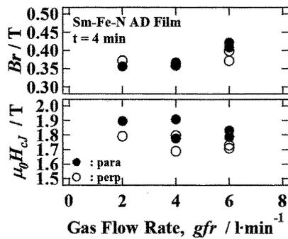
Fig.7 Magnetic properties of Sm-Fe-N AD films deposited with  $gfr = 2-6$  l/min for 4min.
