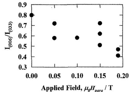
Fig. 14 The variation of  $I_{(006)}/I_{(033)}$  taken from the Sm-Fe-N AD films deposited with  $\mu_0 H_{para}$  of 0-0.19 T.
