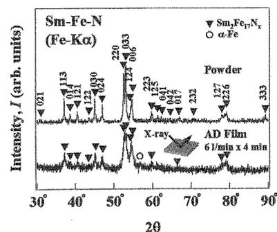
Fig.10 The XRD pattern of the Sm-Fe-N AD film prepared with  $gfr = 6$  l/min and  $t = 4$  min in comparison with that of host powder.
