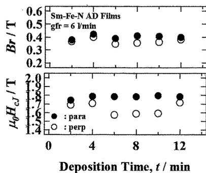
Fig. 8 Magnetic properties of the Sm-Fe-N AD films prepared under the conditions of  $gfr=6$  l/min and  $t=2-12$  min.
