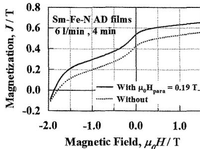
Fig. 12 The demagnetization curves of Sm-Fe-N AD film deposited with or without  $\mu_0 H_{para}$ .
