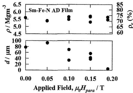
Fig. 11 Variation of thickness ( $d$ ), density ( $\rho$ ) and relative density ( $\rho_r$ ) of the Sm-Fe-N AD films deposited with  $\mu_0 H_{para}$ .
