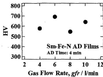
Fig. 3 Vickers hardness of the SmFe-N AD film deposited for 4 min.
