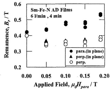
Fig. 13 The  $B_r$  of the Sm-Fe-N AD films deposited with  $\mu_0 H_{para}$  of 0-0.19 T. The films were measured in parallel (para. (in plane)) or perpendicular (perp. (in plane) and perp.) to the direction of  $\mu_0 H_{para}$ .
