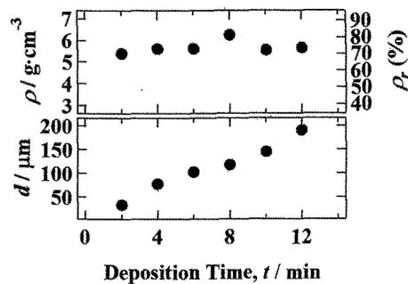
Fig. 5 Variation of thickness ( $d$ ), density ( $\rho$ ) and relative density ( $\rho_r$ ) of Sm-Fe-N AD films as a function of deposition time ( $t$ ).
