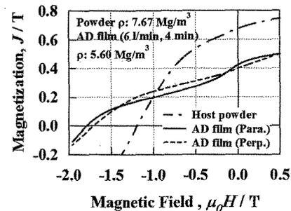
Fig. 6 The demagnetization curve of the Sm-Fe-N AD film deposited with  $gfr = 6$  l/min for 4 min in comparison with that of the host powder.
