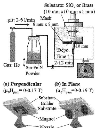
Fig.1 Schematic illustration and conditions of AD method in this study.
