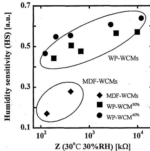
Fig. 4 Relationship between humidity sensitivity and impedance for WP-WCMs and MDF-WCMs at humidity of 30%RH.
