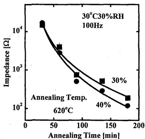
Fig. 2 Annealing time dependence of impedance for WP-WCMs.
