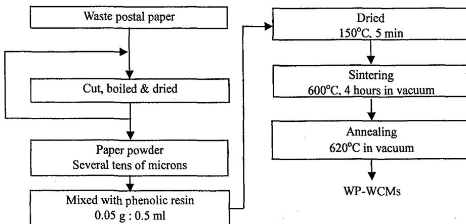
Fig. 1 Fabrication process for WP-WCMs
